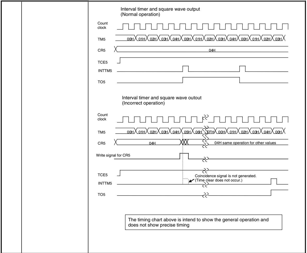
The timing chart above is intend to show the general operation and does not show precise timing
