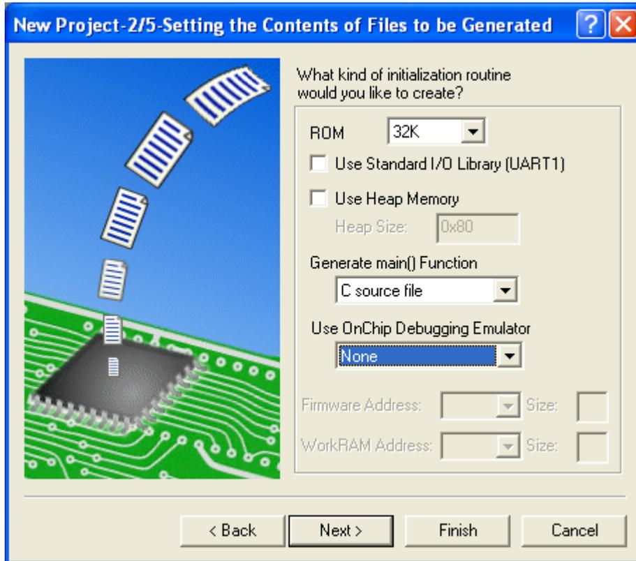
Select the MCU ROM size and heap size. Select “None” for the on-chip debugging emulator. And press [Next].
