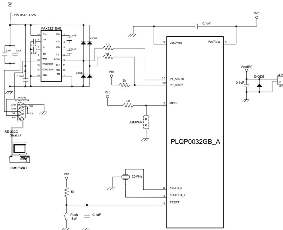
Figure 2 Circuit Using the RS-232C Cable (R8C/2K, 2L Groups)
