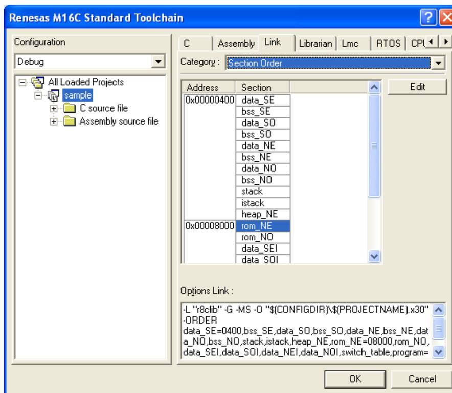
When the user program overlaps with the monitor program occupied area due to the above settings, an error is output.
