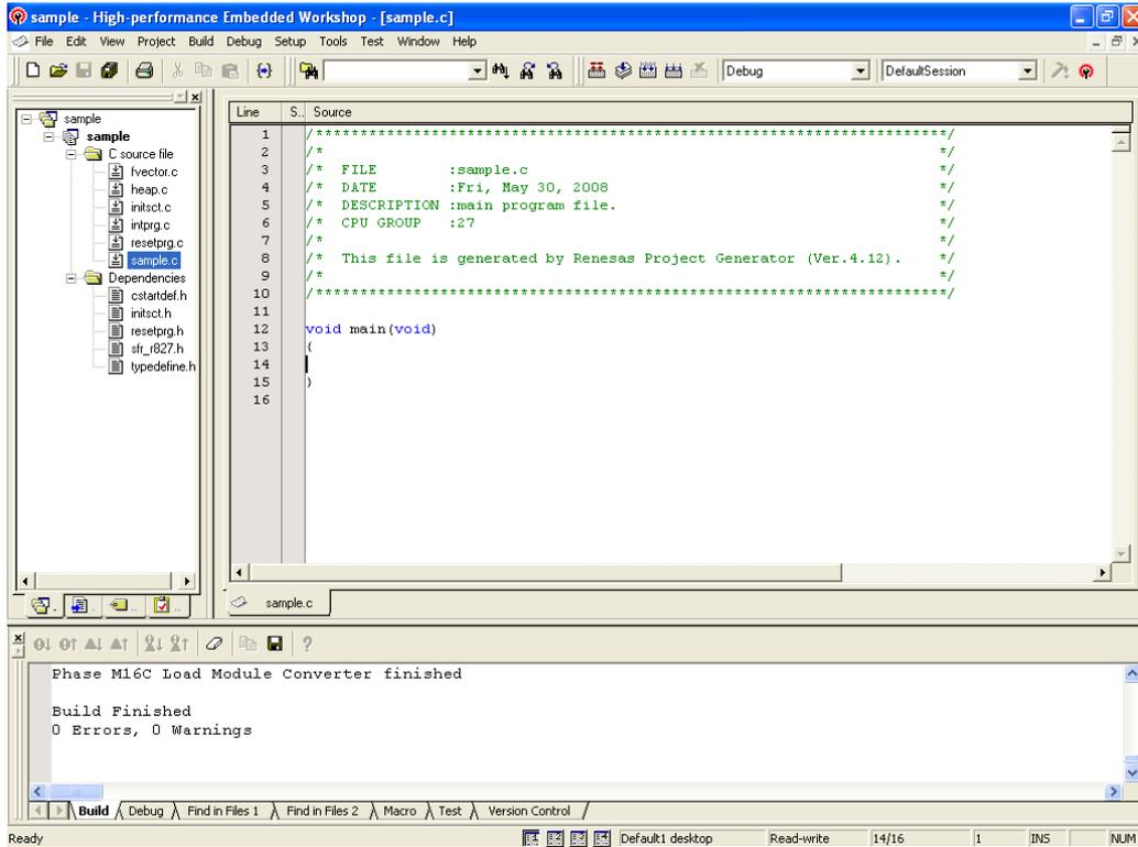
p) Connect with the target. A host computer can be connected with the target easily by switching to the session file in which the setting to use the R8C UART debugger is pre-registered.
