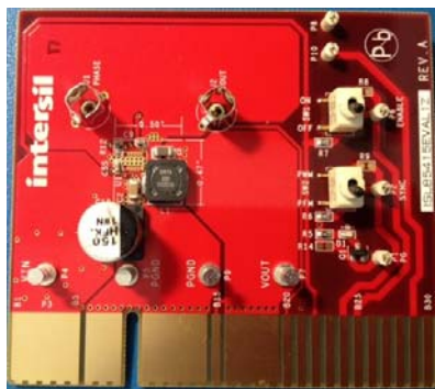
FIGURE 1. FRONT OF EVALUATION BOARD ISL85415EVAL1Z
