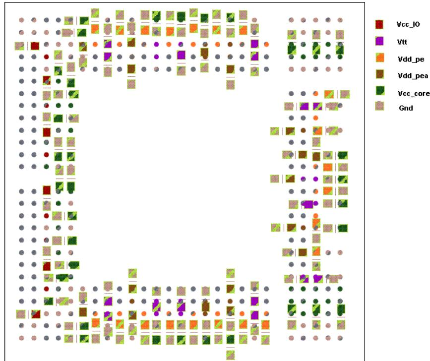
Figure 8 Bypassing Scheme Example Based 0.1nF 0402 Caps
