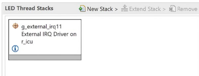
Figure 9-3: The grey color bar of the stack element indicates that this driver is a module instance and that it may be referenced by one other Synergy module instance only
