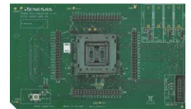
Board dimensions: 160 mm x 100 mm
