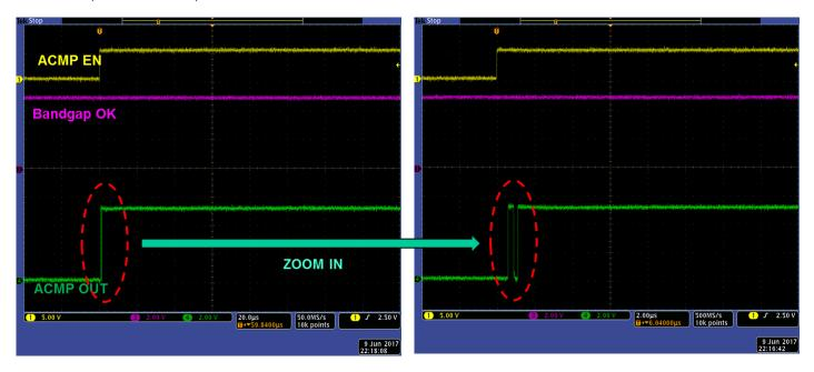
Because BG\_OK is already released by LDO, there is no gating signal. Depending on the ACMP VREF condition & the positive input value, it is possible for the ACMP to have a glitch. Subsequently, the other ACMP will not have an issue unless the customer repeats LDO enable first and ACMP later during power stable.
