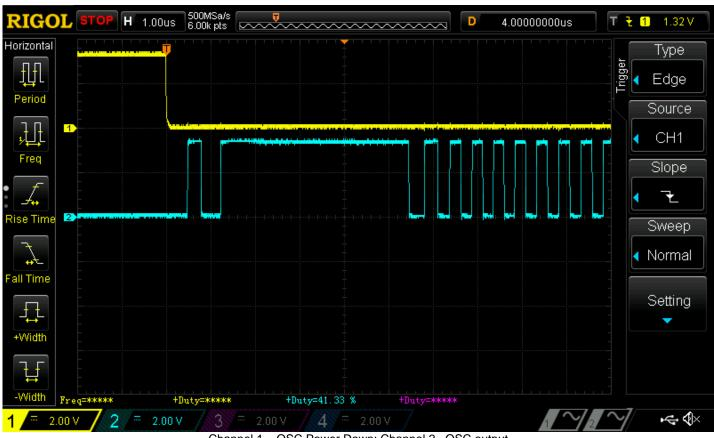
Channel 1 - OSC Power Down; Channel 2 - OSC output
