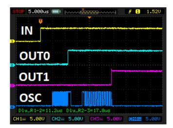
If there are some inner blocks which use RC OSC at the moment or RC OSC is forced power on when such error appears, RC OSC will be operational and delay value will be proper.
