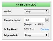
The configuration shown above generates a periodical signal with a frequency defined by the Delay cell and started by a HIGH signal on PIN2. The issue becomes apparent in a longer settling time when the scheme generates short pulses (Delay is configured as a rising edge delay only). See waveform below.
