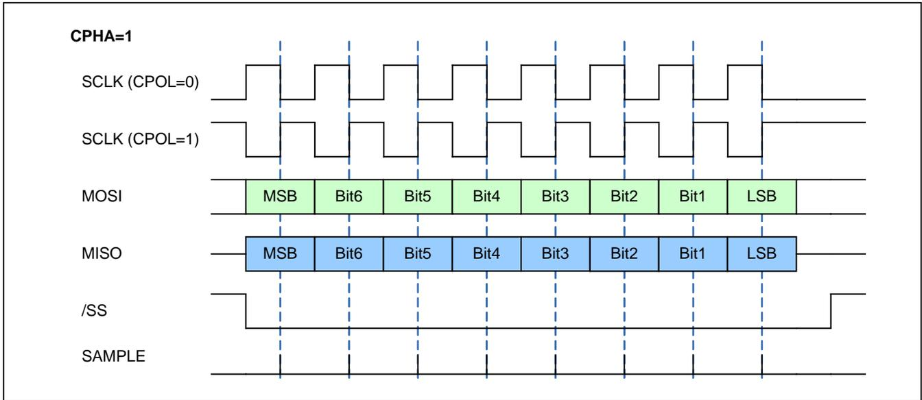
In SPI mode, each command except NOP is started as shown in Figure 3.5. After the execution of a command (busy = 0), the expected data can be read as illustrated in Figure 3.6 or if no data are returned by the command, the next command can be sent. The status can be read at any time with the NOP command (see Figure 3.7).
