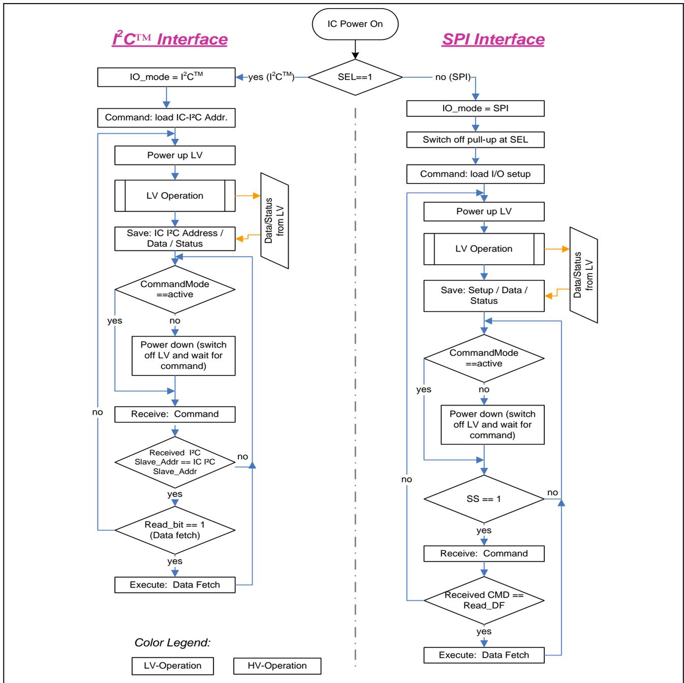
Figure 3.2 Operational Flow Chart: Command Mode and Normal Mode
