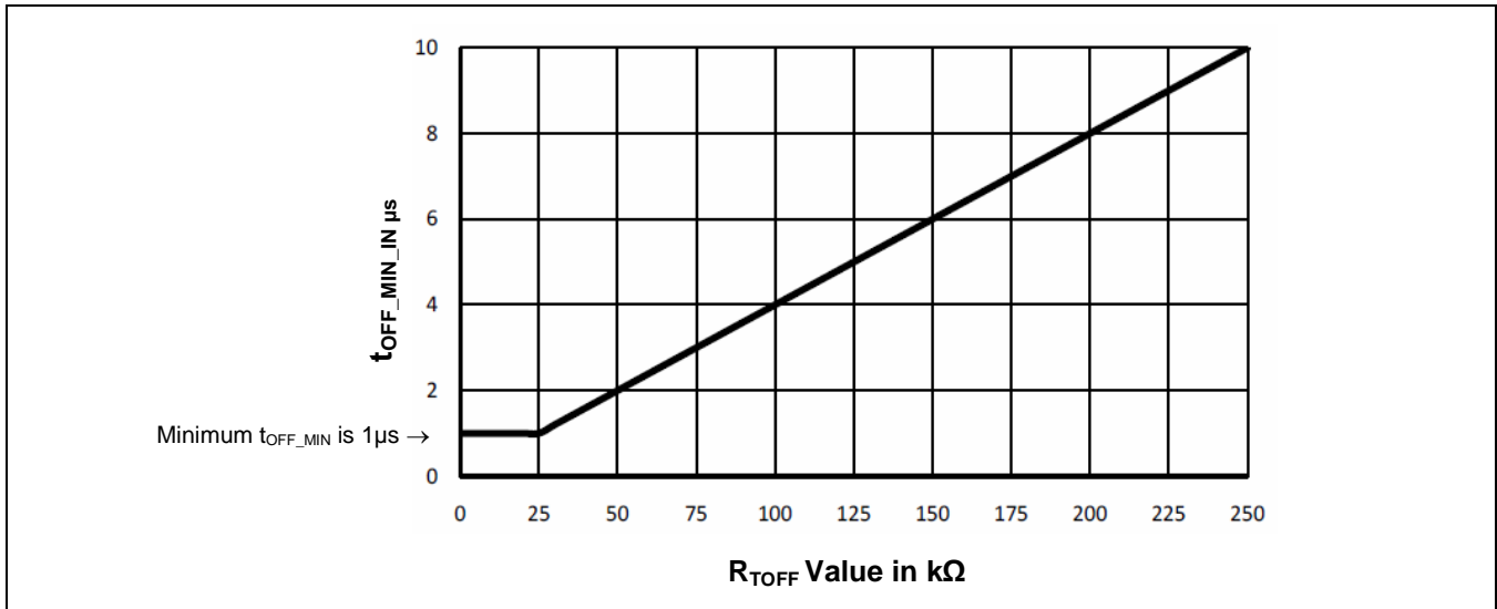
Figure 2.5 Minimum Off-Time t_{OFF\_MIN} vs. R_{TOFF}
