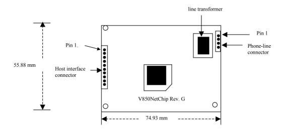
Figure 1: Outline plan (component side) of V850NetChip-ISDN
