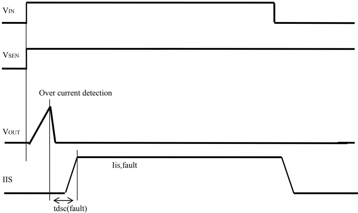
Fault signal delay time at power limitation
