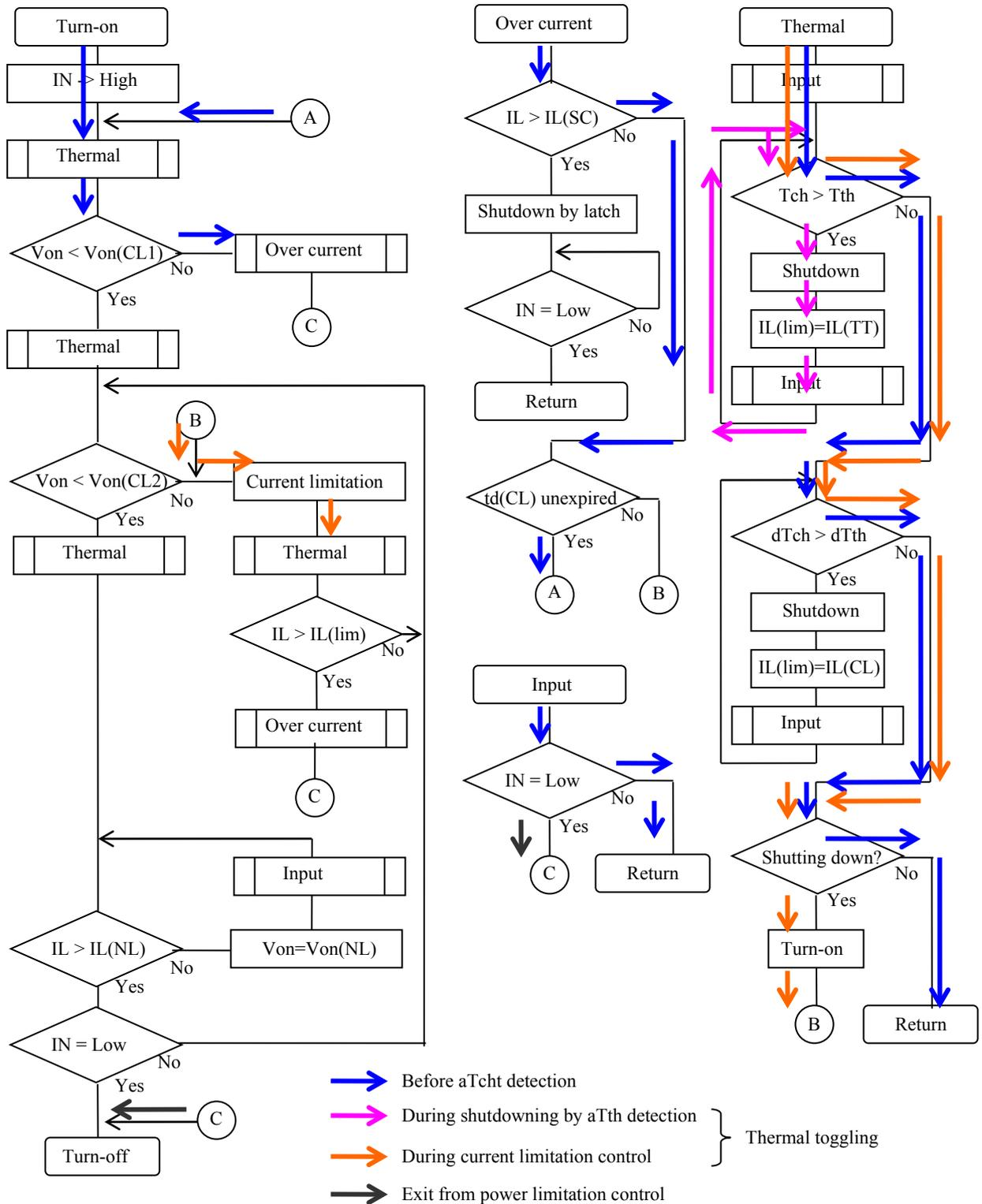
An over load condition which is include a short circuit condition during on-state
