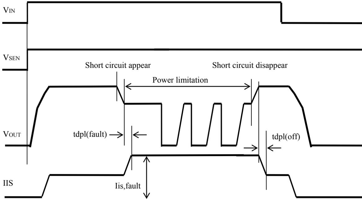
Fault signal delay time at Thermal toggling
