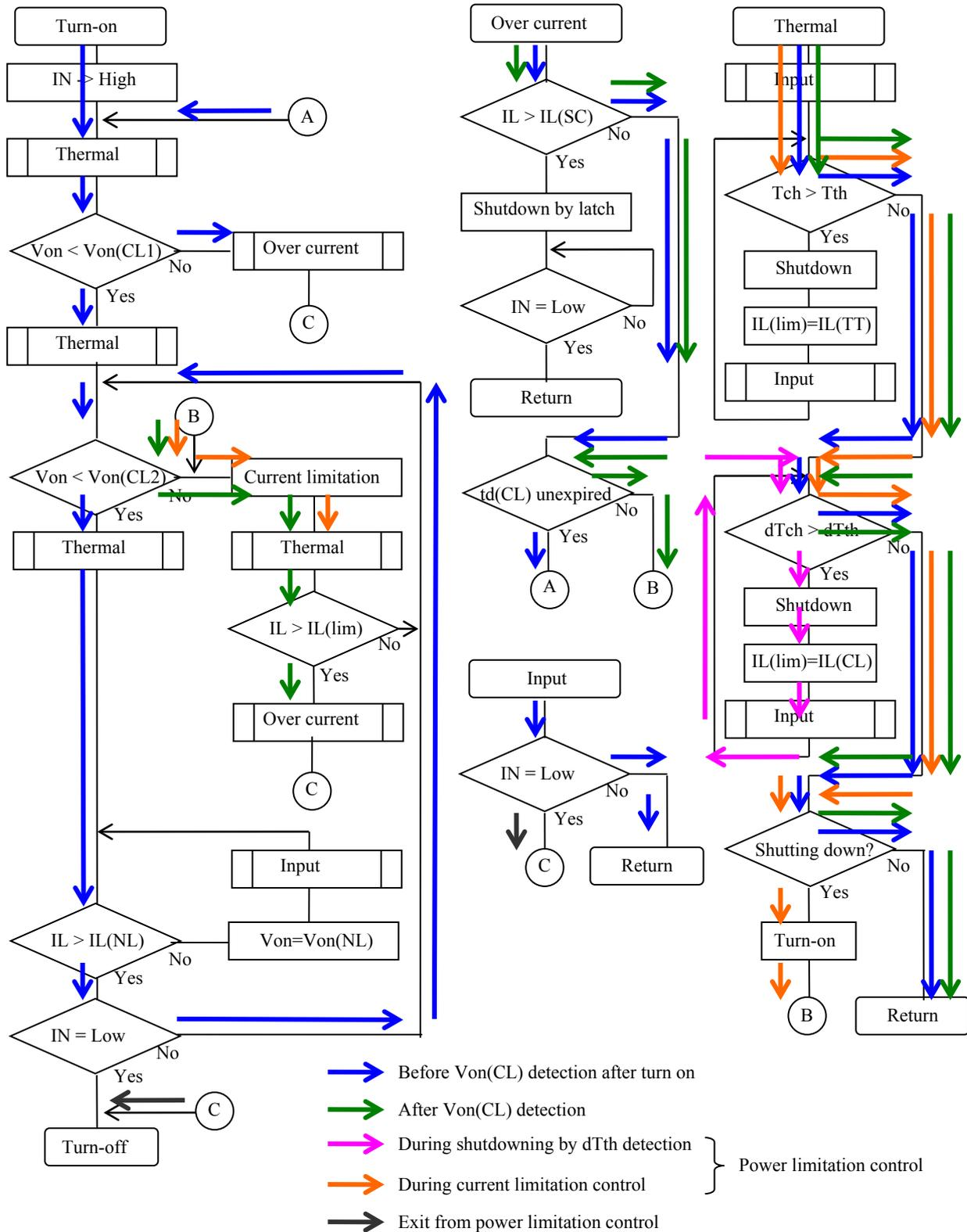
An over load condition including short circuit condition during on-state
