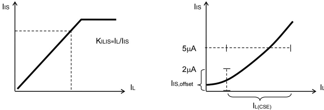
**Sense current under fault condition**
