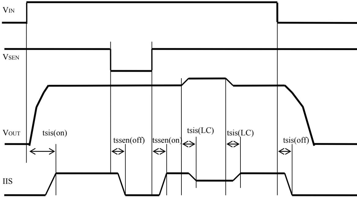
Fault signal delay time at over current detection
