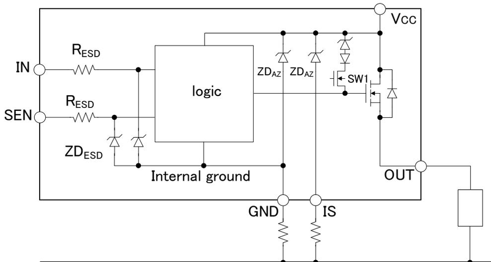
**3.6.2 Device behavior at over voltage condition**
