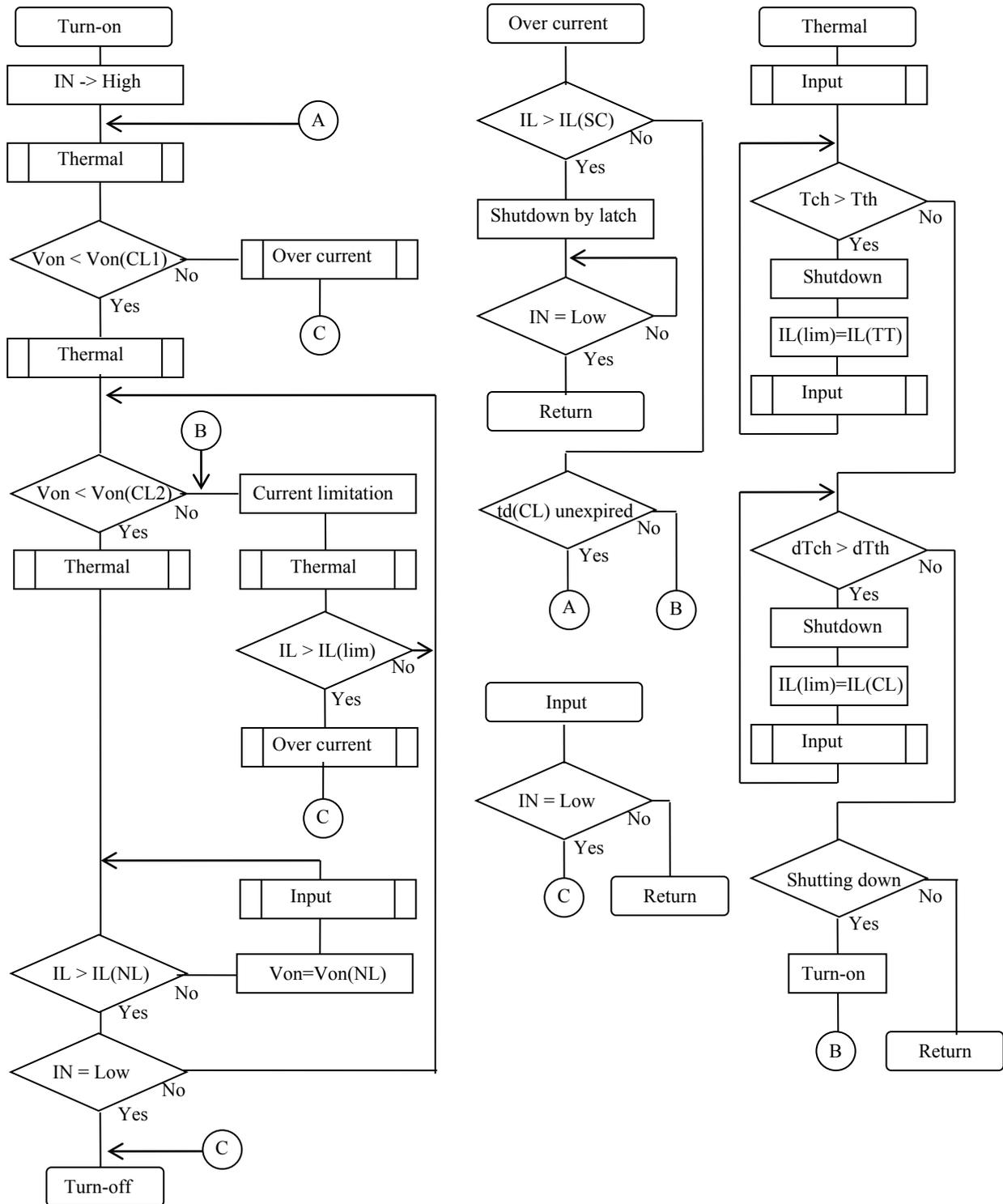
Turn-on in an over load condition including short circuit condition
