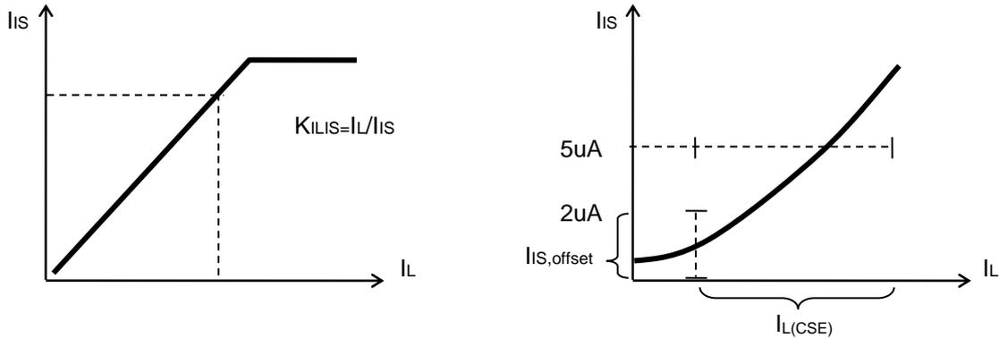
**Sense current under fault condition**
