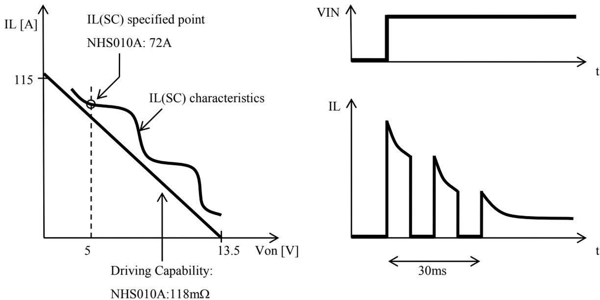
**3.6.10 Cross current protection in case of H-bridge high side usage**
