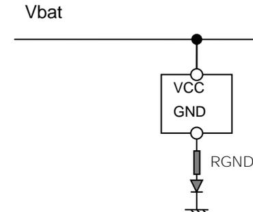
External diode and resistor are recommended in order to prevent reverse current toward control logic part at reverse battery condition and limit the current through ZD<sub>AZ</sub> at load dump condition. 100Ω is recommended as RGND.
