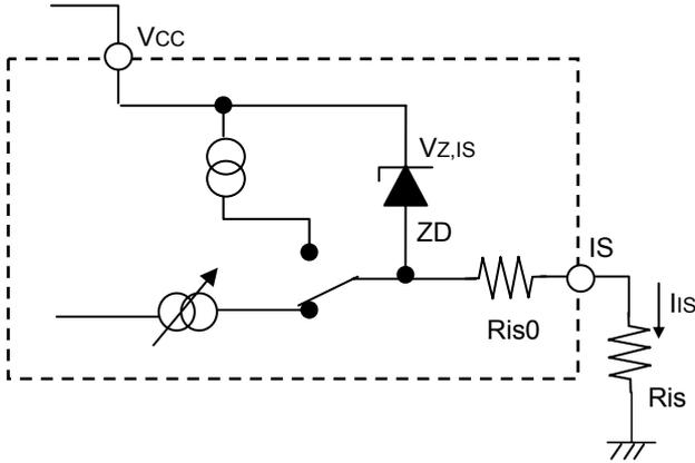
Ris0 is 130 Ω typ.  $V_{z,IS} = 46\text{ V (typ.)}$ ,  $R_{IS} = 1\text{ k}\Omega$  nominal.  $I_S$  can be only driven by the internal circuit as long as  $V_{IS} < V_{out} - 6\text{ V}$ .  $R_{IS}$  should be less than 20 kΩ for any application. Even If current sense and diagnostic features are not used,  $R_{IS}$  has to be connected.
