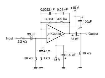
TYPICAL CHARACTERISTIC Distortion 0.03% (Vo =  $1V_{r.m.s.}$ , f = 1 kHz)
