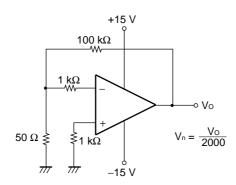
Figure 2 Channel Separation Measurement Circuit
