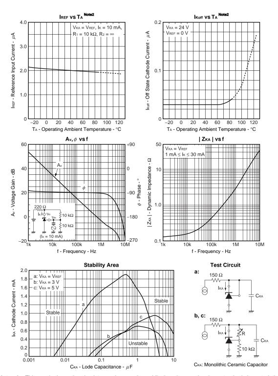
Notes 1. This graph shows the absolute maximum rating, while the other graphs show standard characteristics. Be sure to use the devices within the ranges delimited by the solid lines shown for each device.
