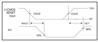
Voltage and Current Waveforms Inputs Active and Inactive
