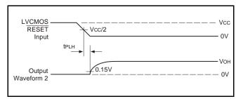
Voltage Waveforms: Open Drain Output Low-to-High Transition Time (with respect to RESET input)
