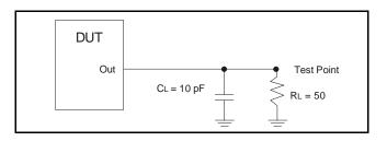
Load Circuit: Low-to-High Slew-Rate Adjustment
