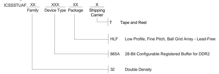
ICSSSTUAF32865A 28-BIT CONFIGURABLE REGISTERED BUFFER FOR DDR2
