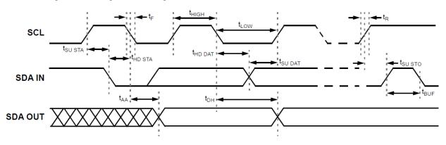
Figure2. I2C Serial General Timing
