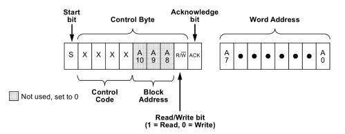
Figure 1. I2C Basic Command Structure
