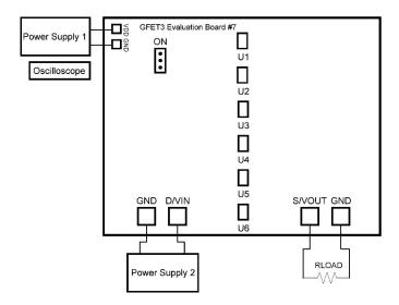
Figure 3. Typical connections for GreenFET Evaluation.
