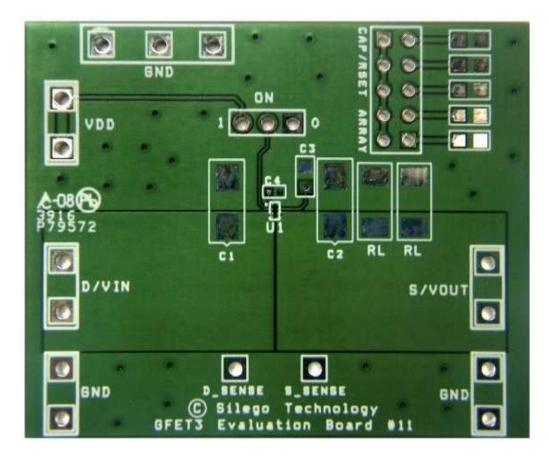
Figure 5. SLG59M1735C Evaluation Board
