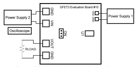
Figure 10. SLG59M1717V Evaluation Board Connection Circuit
