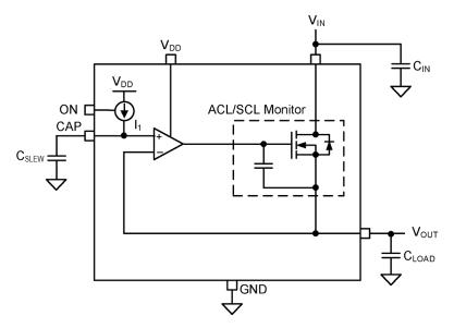
Figure 5. SLG59M1717V's Equivalent Slew-rate Control Loop Circuit
