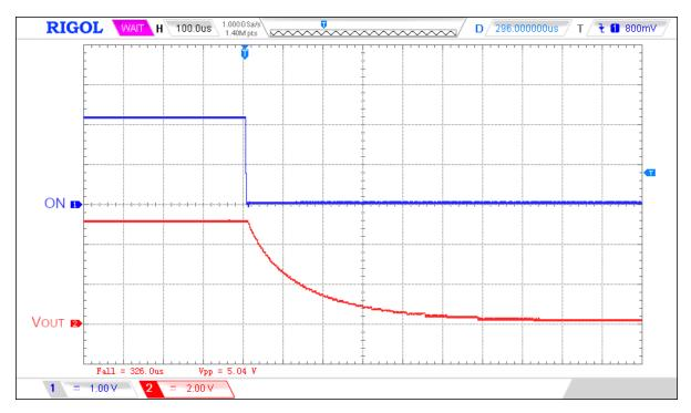
Figure 4. Typical Turn OFF operation waveform for  $V_{DD}$  =  $V_{D}$  = 5 V,  $C_{SLEW}$  = 12 nF,  $C_{LOAD}$  = 10  $\mu$ F,  $R_{LOAD}$  = 20  $\Omega$
