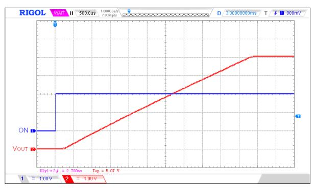
Figure 7. A SLG59M1717V with  $C_{SLEW}$  set to 15nF and 470 $\mu$ F retained for  $C_{LOAD}$ .  $C_{LOAD}$ -to- $C_{SLEW}$  ratio is smaller than 33,600. Note smooth  $V_{OUT}$  transition.
