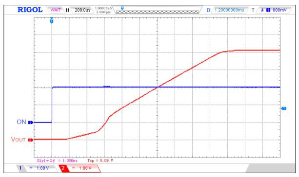
Figure 6. A SLG59M1717V with  $C_{SLEW}$  set to 4nF and 470 $\mu$ F for  $C_{LOAD}$ .  $C_{LOAD}$ -to- $C_{SLEW}$  ratio is greater than 33,600. Note that the internal SCL monitor's been triggered and  $V_{OUT(SR)}$  is reduced until  $V_{OUT}$  reaches ~0.25V.
