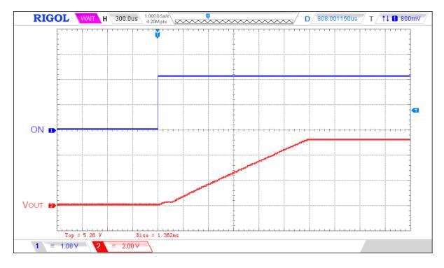
Figure 2. Typical Turn ON operation waveform for  $V_{DD}$  =  $V_D$  = 5 V,  $C_{SLEW}$  = 4 nF,  $C_{LOAD}$  = 10  $\mu$ F,  $R_{LOAD}$  = 20  $\Omega$
