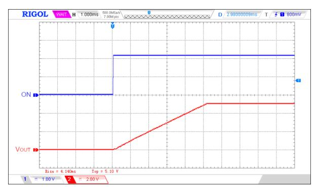
Figure 1. Typical Turn ON operation waveform for  $V_{DD}$  =  $V_D$  = 5 V,  $C_{SLEW}$  = 12 nF,  $C_{LOAD}$  = 10  $\mu$ F,  $R_{LOAD}$  = 20  $\Omega$
