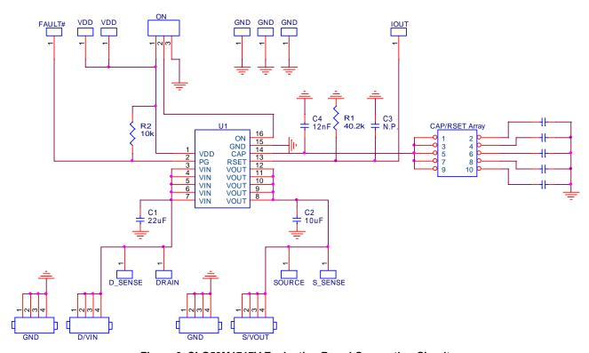
Figure 9. SLG59M1717V Evaluation Board Connection Circuit
