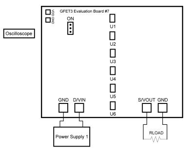
Figure 3. Typical connections for GreenFET Evaluation.
