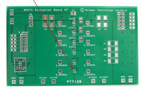
Figure 1. SLG59M1440V Evaluation Board.
