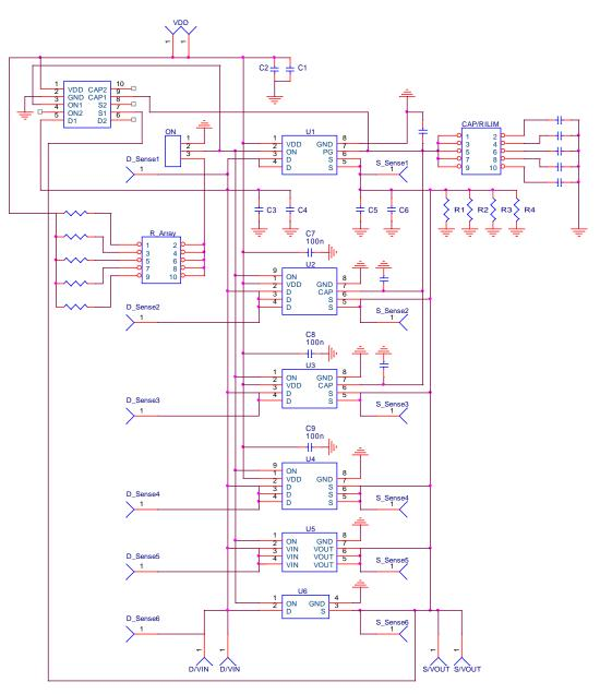
Figure 2. SLG59M1440V Evaluation Board Connection Circuit.
