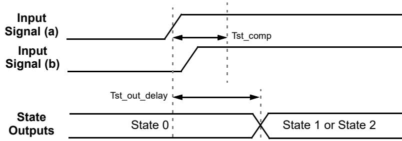
Figure 95. State Transition Timing - Competing Inputs Indeterminate
