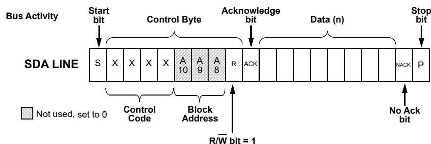
**Figure 105. Current Address Read Command, R/W = 1**
