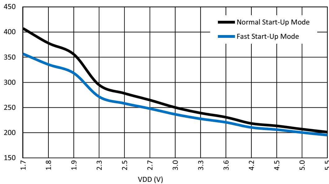
Figure 71. RC Oscillator Maximum Power On Delay vs. V<sub>DD</sub> at room temperature, OSC0 = 2 MHz
