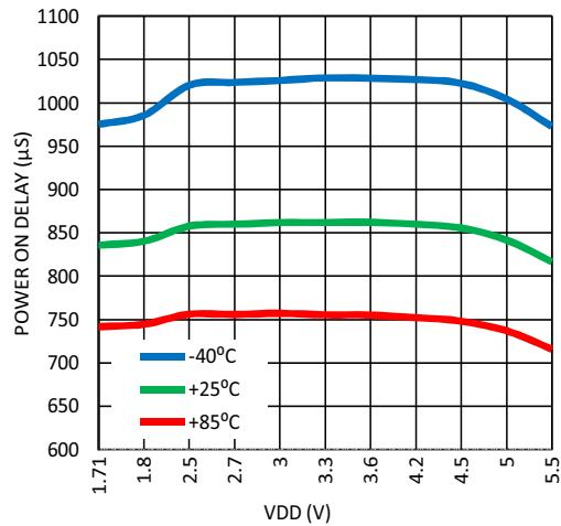
**Figure 52. Maximum Power On Delay vs.  $V_{DD}$ ,
