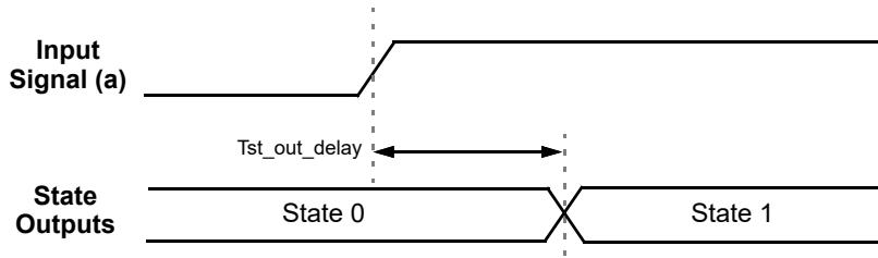
Figure 89. State Transition Timing
