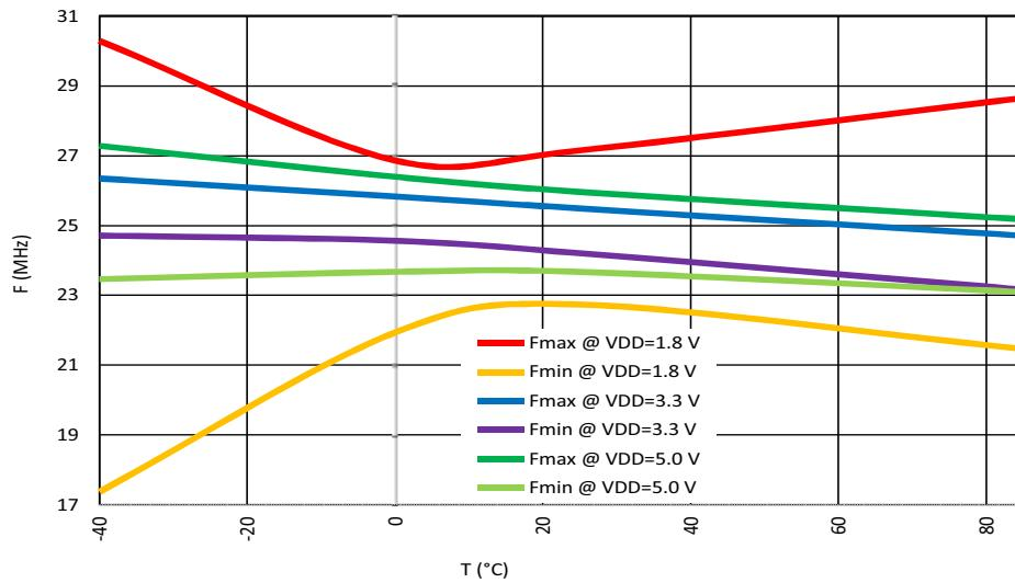
**Figure 76. OSC1 (25 MHz) Frequency vs. Temperature**
