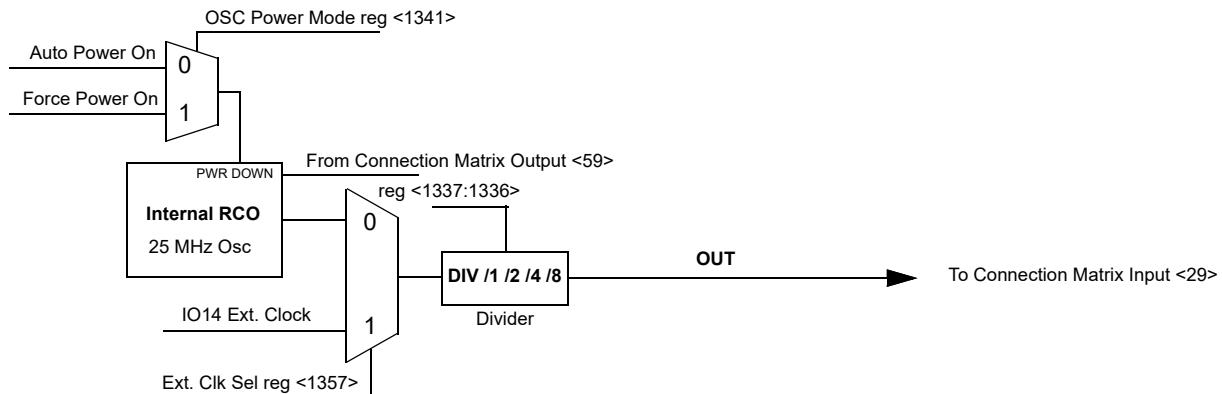
Figure 69. 25 MHz RC OSC Block Diagram
