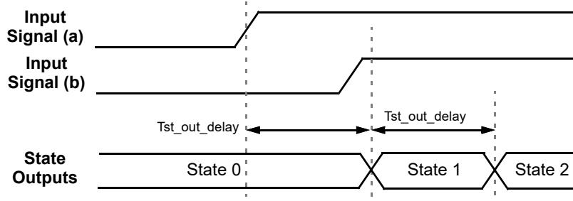
Figure 98. State Transition - Sequential Timing
