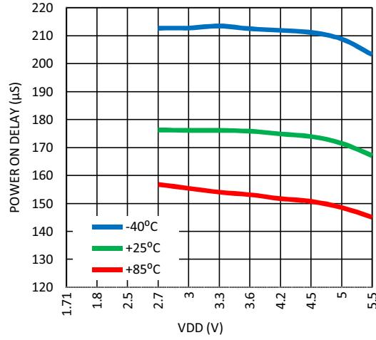
**Figure 53. Maximum Power On Delay vs.  $V_{DD}$ ,
