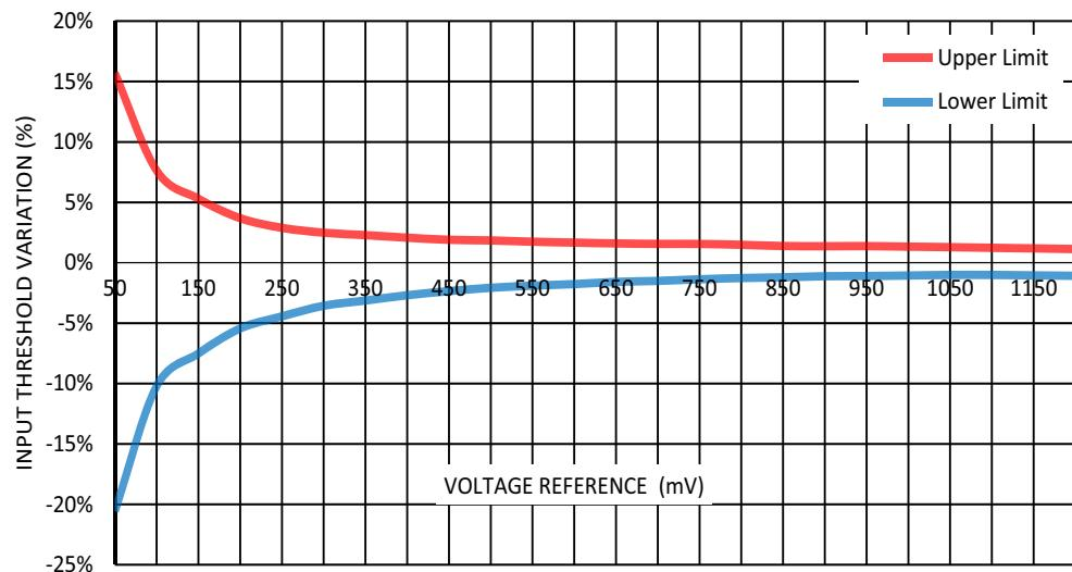
**Figure 55. Typical Input Threshold Variation (including Vref variation, ACMP offset) vs. Voltage Reference at  $T = (-40.... +85)^\circ\text{C}$ , LMB Mode - Disable,  $V_{\text{phys}} = 0 \text{ mV}$ .**
