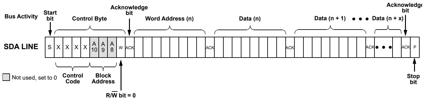
**Figure 104. Sequential Write Command, R/W = 0**
