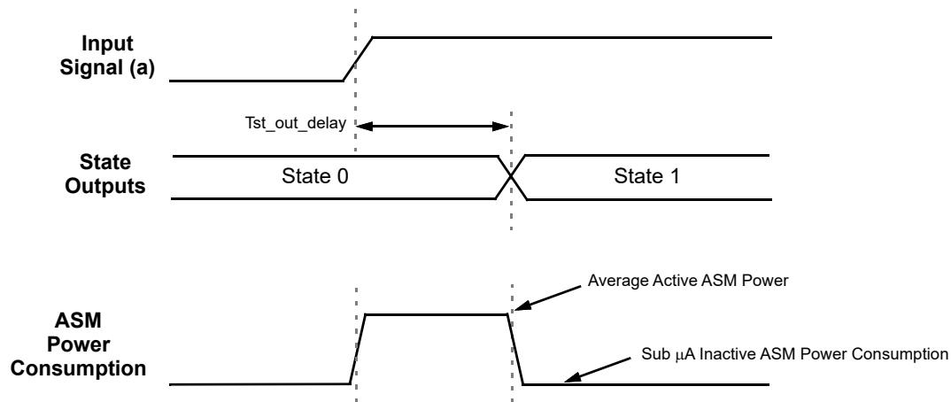
**Figure 91. State Transition Timing and Power Consumption**
