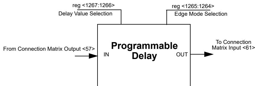
Figure 60. Programmable Delay
