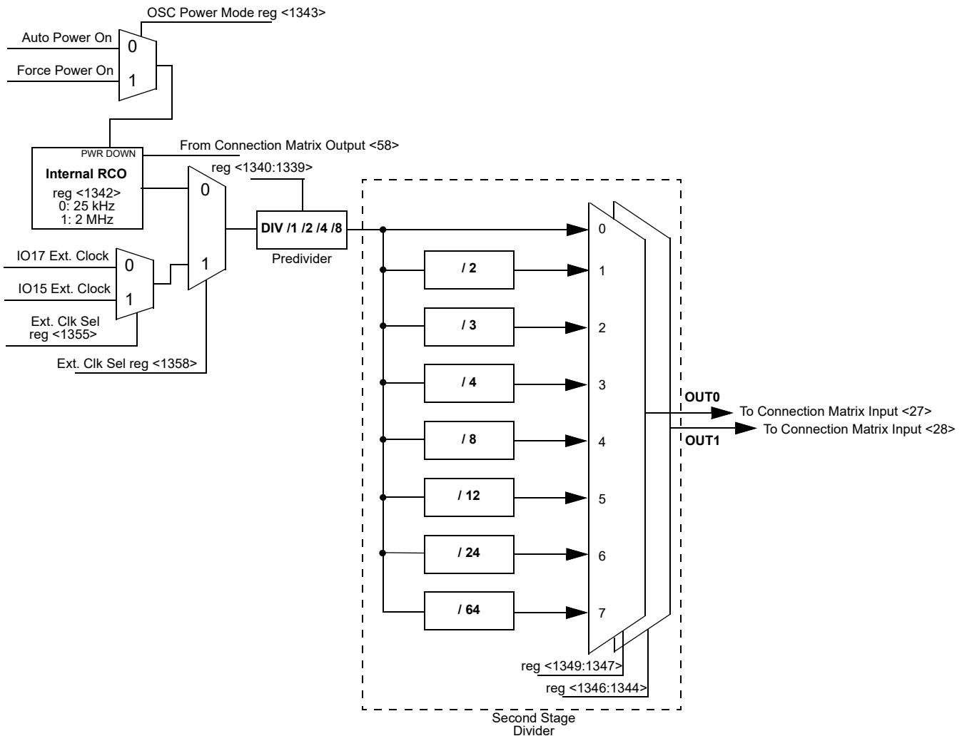
Figure 68. 25 kHz / 2 MHz RC OSC Block Diagram
