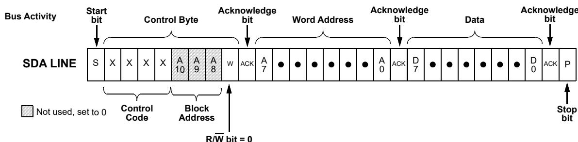
**Figure 103. Byte Write Command, R/W = 0**
