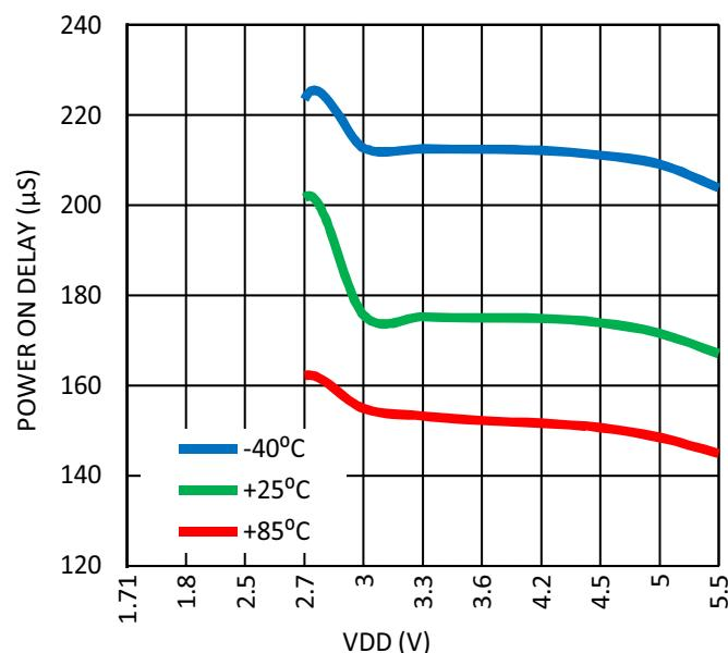
**Figure 51. Maximum Power On Delay vs.  $V_{DD}$ ,
