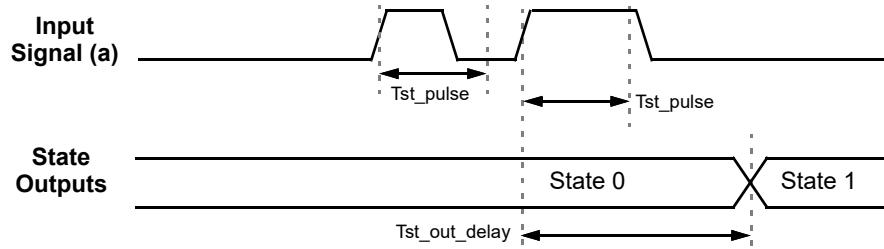
Figure 93. State Transition Pulse Input Timing
