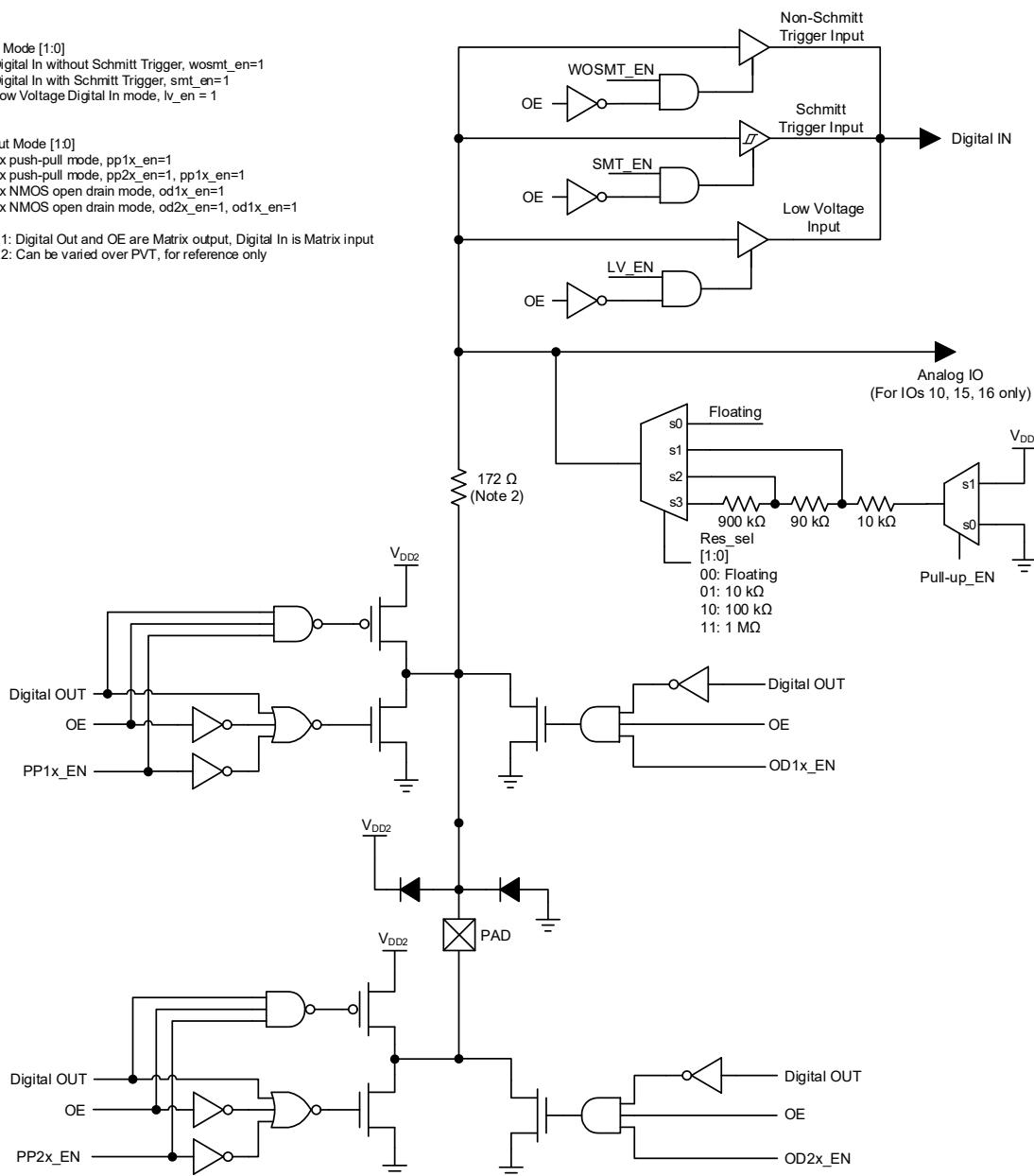
Figure 4. Matrix OE IO Structure Diagram
