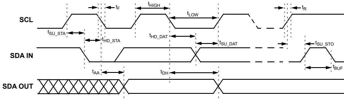
**Figure 102. I<sup>2</sup>C General Timing Characteristics**
