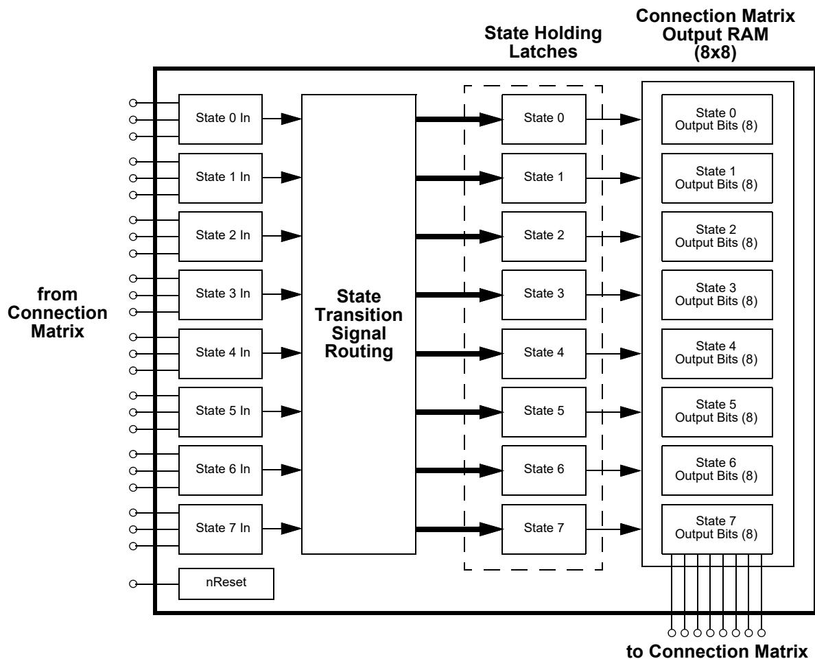
Figure 83. Asynchronous State Machine
