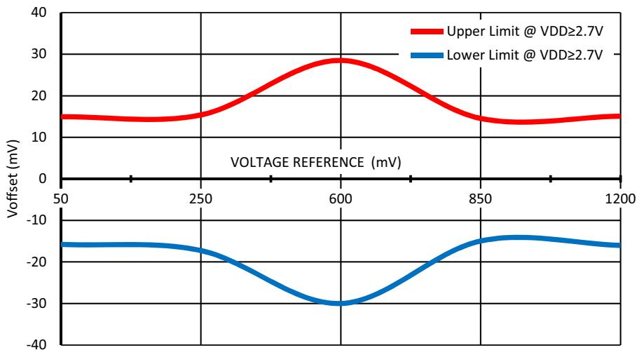
**Figure 54. Typical Buffer Input Voltage Offset vs. Voltage Reference at  $T = (-40....+85)^\circ\text{C}$ ,
