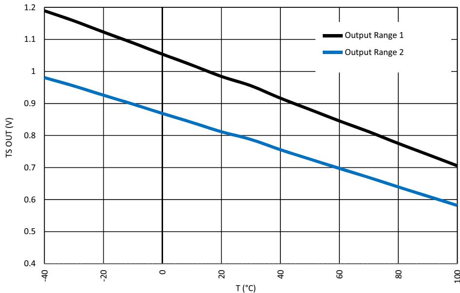
Figure 111. TS Output vs. Temperature,  $V_{DD} = (1.71 \dots 5.5) \text{ V}$
