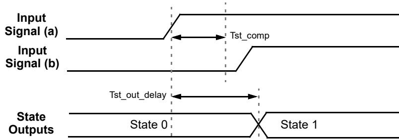
Figure 96. State Transition Timing - Competing Inputs Determinable
