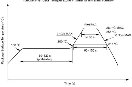
JEDEC J-STD-020E compliant soldering conditions
