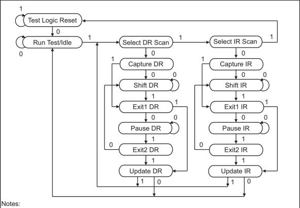
The value adjacent to each state transition in this figure represents the signal present at TMS at the time of a rising edge at TCK.
