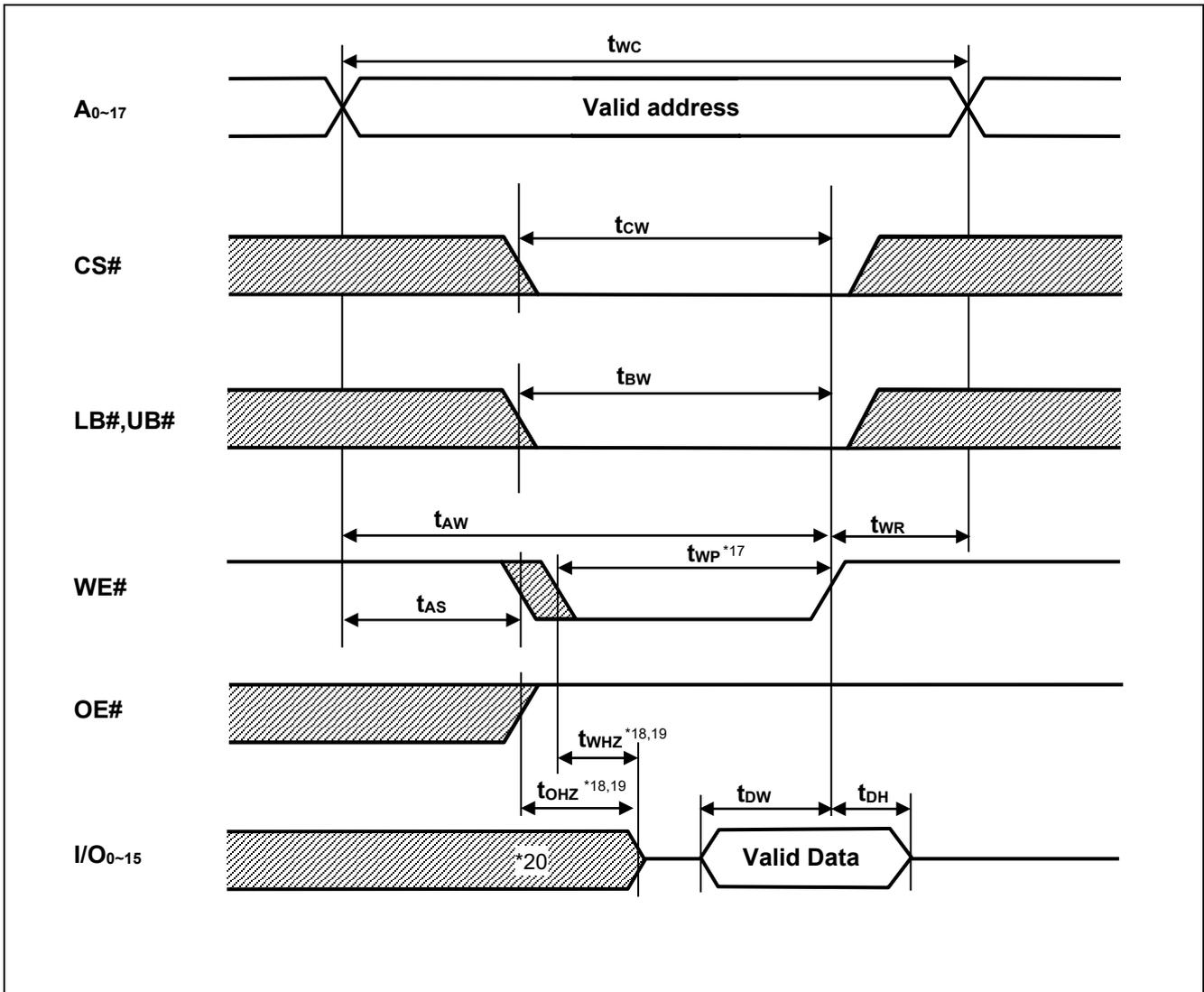
Note 17.  $t_{WP}$  is the interval between write start and write end.
