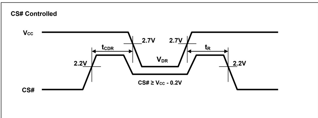
Low V<sub>CC</sub> Data Retention Timing Waveforms (LB#,UB# controlled)
