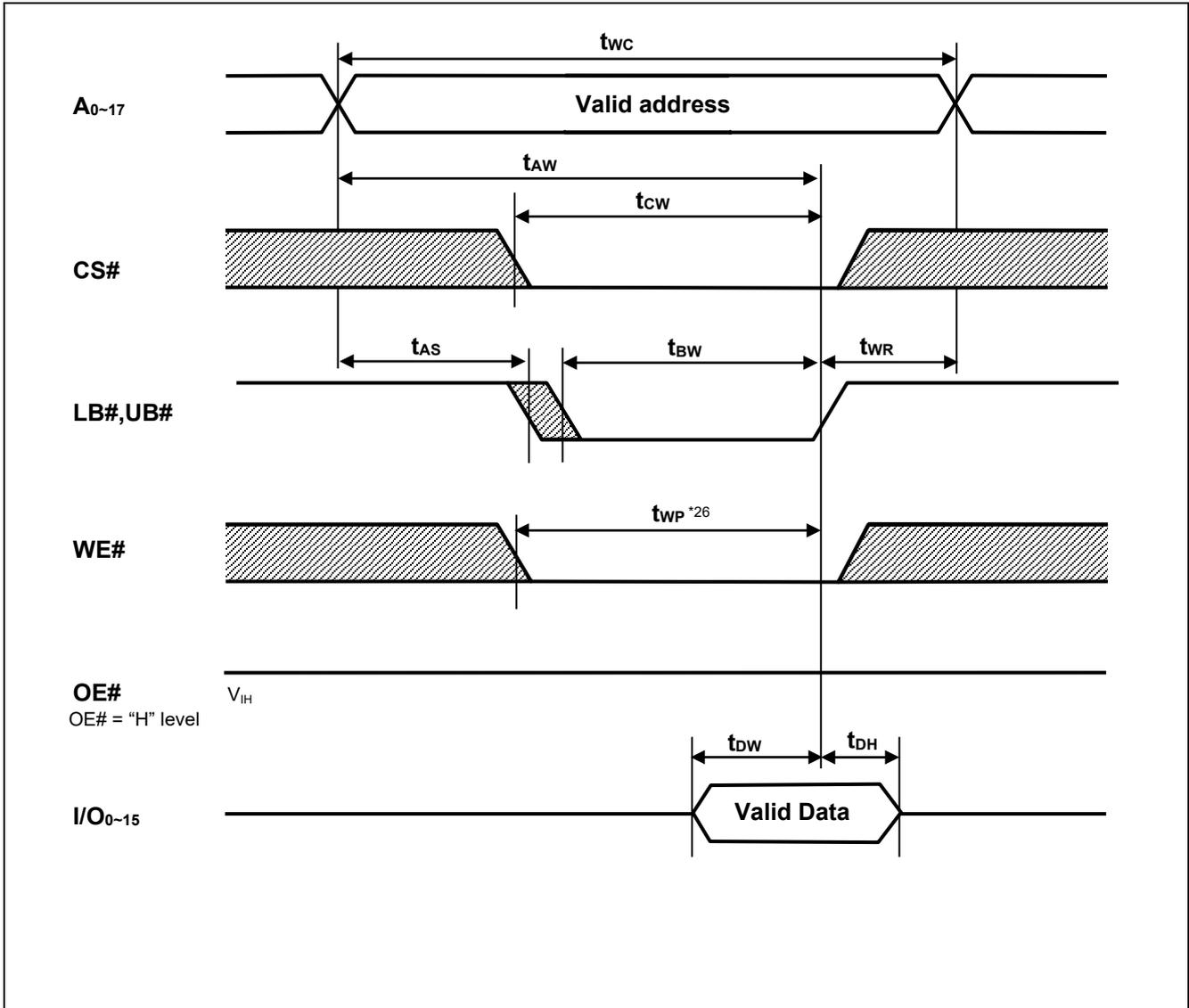
Note 26.  $t_{WP}$  is the interval between write start and write end.
