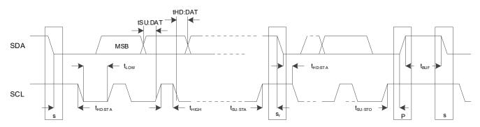
Figure 4. I<sup>2</sup>C Slave Timing Diagram
