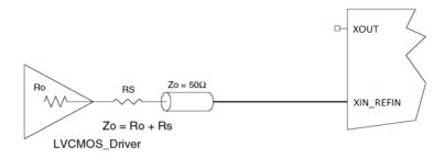
Figure 7. 1.2V LVCMOS Driver to XTAL Input Interface
