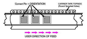
Figure 15. Pin 1 Orientation in Tape and Reel Packaging
