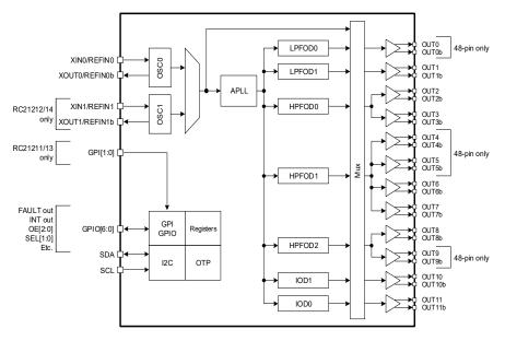
Figure 1. RC2121xA Block Diagram
