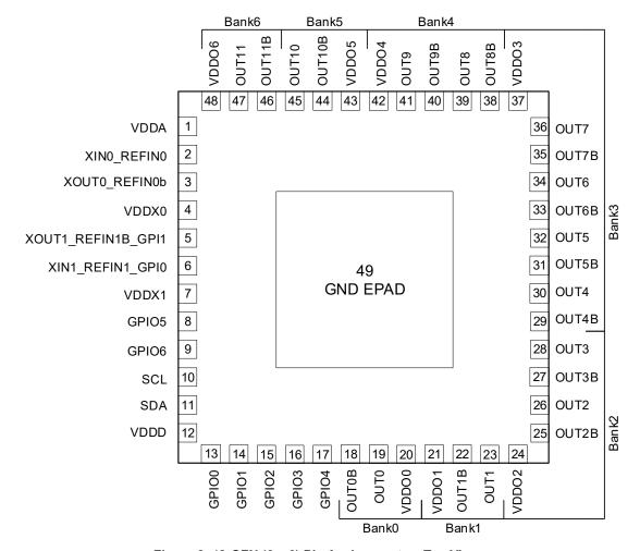
Figure 2. 48-QFN (6 × 6) Pin Assignments – Top View
