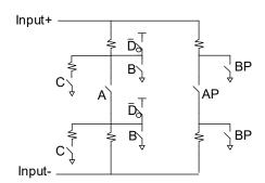
Figure 5. Programmable Input Buffer Logical Diagram
