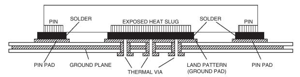
Figure 14. P.C. Assembly for Exposed Pad Thermal Release Path - Side View (Drawing not to Scale)
