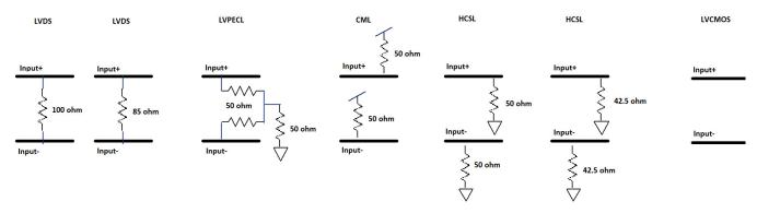
Figure 6. Input Buffer Behavior by Protocol
