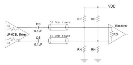
Figure 12. AC-Coupling Termination
