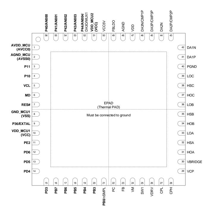
Figure 4.2-1 Pin Configuration Diagram (Top View)
