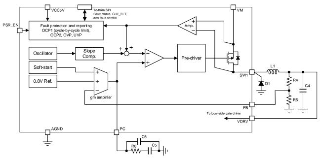
Figure 6.3-2 Buck Regulator Block Diagram
