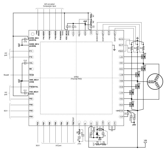
Figure 8-1 External Circuit Example - 3 Shunt Sensorless FOC
