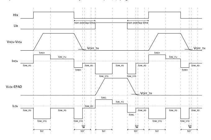
Figure 6.4-2 Gate Drive Timing Diagram in 3-Phase HI/LI Mode if the HI/LI Inserted Dead Time is Relatively Long
