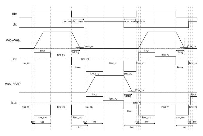
Figure 6.4-4 Gate Drive Timing Diagram with DIS\_SADT=1 if the HI/LI Inserted Dead Time is Shorter than Gate Transition Time
