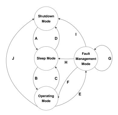
Figure 6.1-2 Mode Transition State Machine
