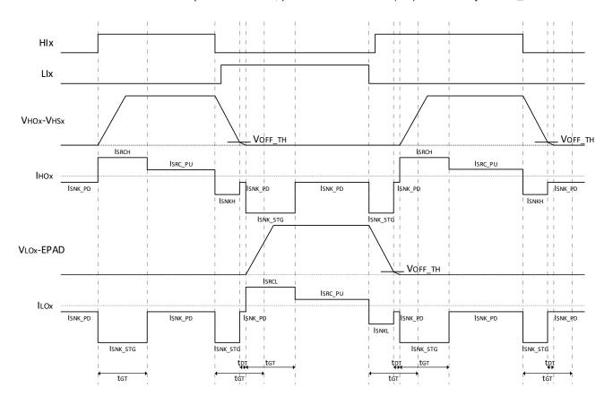
Figure 6.4-3 Gate Drive Timing Diagram in 3-Phase HI/LI Mode if the HI/LI Inserted Dead Time is Relatively Short
