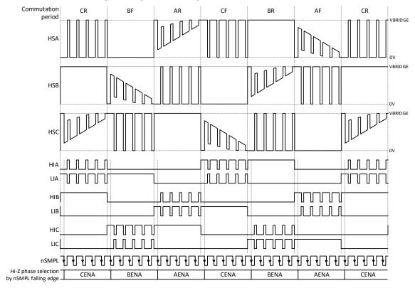
Figure 6.5-3 The Relation Between Typical Six Step Trapezoidal Drive and BEMF Detect Phase
