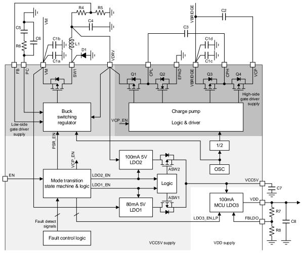
Figure 6.3-1 Block Diagram of Power Supply Blocks
