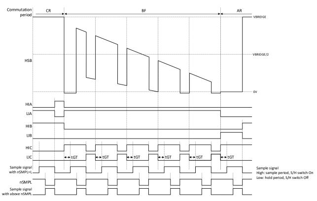
Figure 6.5-4 S/H Timing During Commutation Period BF
