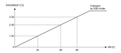
Figure 6.5-6 The Relation Between DA3O/MUX1 and VM Voltage
