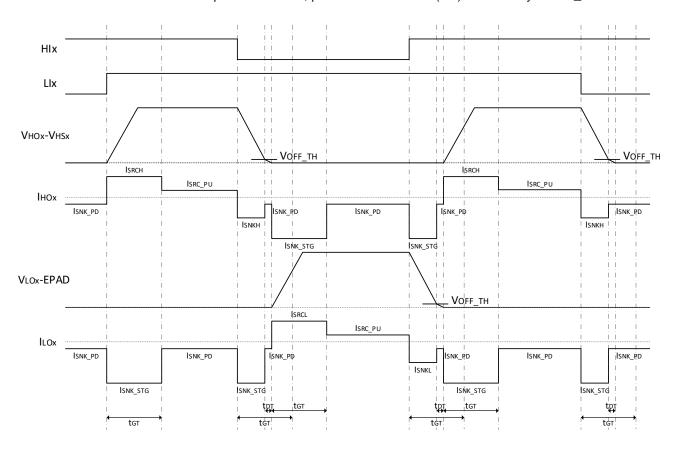
Figure 6.4-6 Gate Drive Timing Diagram in 3-Phase PWM Mode
