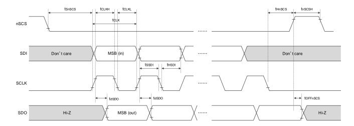
Figure 5.5-1 SPI Timing Diagram
