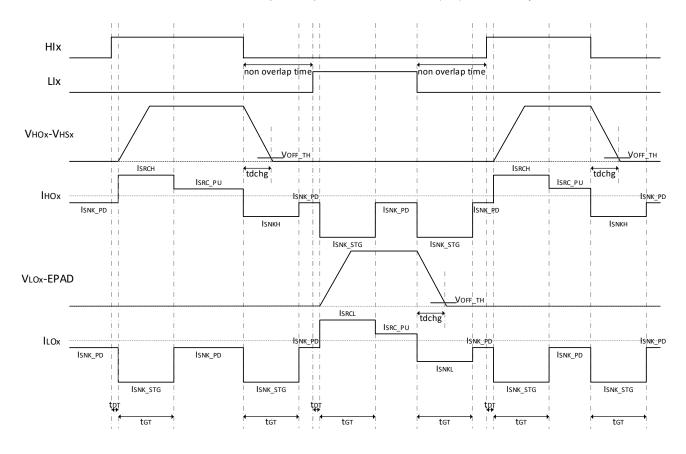
Figure 6.4-5 Gate Drive Timing Diagram with DIS\_SADT=1 if the HI/LI Inserted Dead Time is Longer than Gate Transition Time
