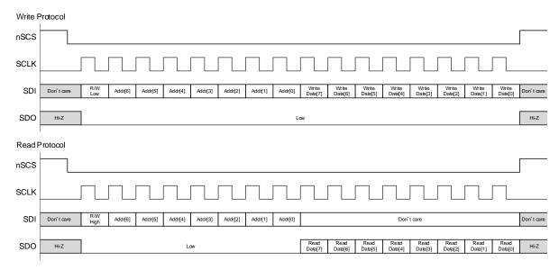
Figure 6.6-1 SPI Communication Format
