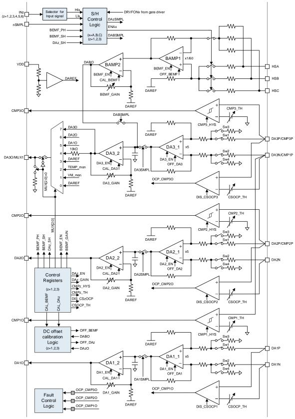
Figure 6.5-1 Block Diagram of Sense Block
