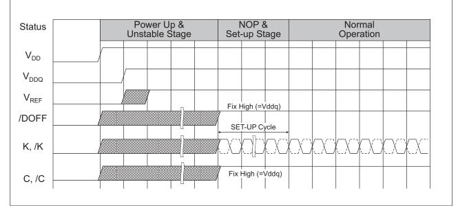
2. Double Clock Mode (C and /C control outputs)
