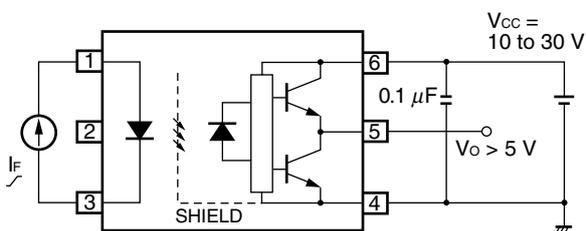
Fig. 6 I<sub>CCH</sub>/I<sub>CCL</sub> Test Circuit
