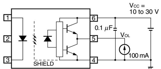
Fig. 5 I<sub>FLH</sub> Test Circuit
