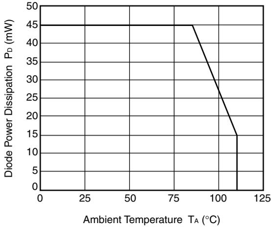
**DETECTOR POWER DISSIPATION vs. AMBIENT TEMPERATURE**
