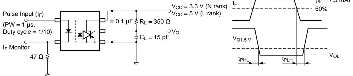
Remark:  $C_L$  includes probe and stray wiring capacitance.
