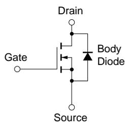
**Remark** Strong electric field, when exposed to this device, can cause destruction of the gate oxide and ultimately degrade the device operation. Steps must be taken to stop generation of static electricity as much as possible, and quickly dissipate it once, when it has occurred.
