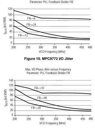
Max. I/O Phase Jitter versus Frequency
