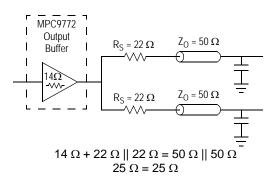
Figure 14. Optimized Dual Line Termination
