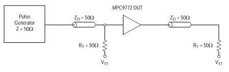
Figure 15. CCLK MPC9772 AC Test Reference
