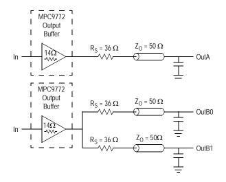
Figure 12. Single versus Dual Transmission Lines
