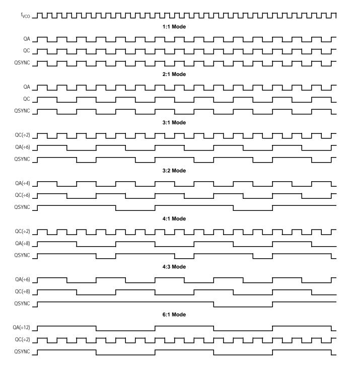
Figure 6. QSYNC Timing Diagram
