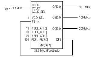
MPC9772 example configuration (feedback of QFB = 33.3 MHz,  $f_{VCO}$ =400 MHz, VCO\_SEL=+1, M=12, N<sub>A</sub>=12, N<sub>B</sub>=4, N<sub>C</sub>=2).
