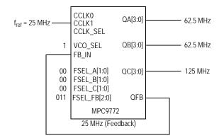
MPC9772 example configuration (feedback of QFB = 25 MHz,  $f_{VCO}$ =250 MHz, VCO\_SEL=÷1, M=10, N<sub>A</sub>=4, N<sub>B</sub>=4, N<sub>C</sub>=2).
