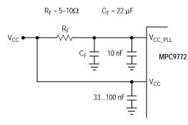
Figure 7. V<sub>CC PLL</sub> Power Supply Filter
