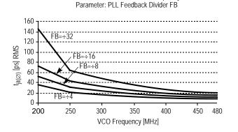
Max. I/O Phase Jitter versus Frequency
