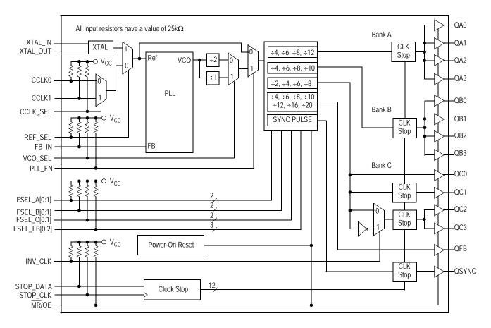
Figure 1. Logic Diagram
