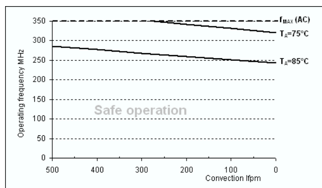
Figure 9. Maximum MPC9443 Frequency, V_{CC} = 3.3 V, MTBF 4 Years, 4 pF Load per Line
