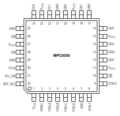
Figure 2. Pinout: 32-Lead Package Pinout (Top View)
