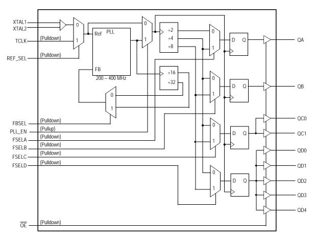
Figure 1. MPC9350 Logic Diagram
