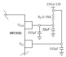
Figure 3. Power Supply Filter
