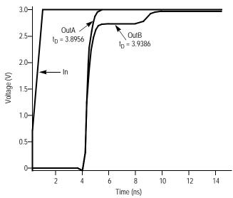
Figure 5. Single versus Dual Waveforms
