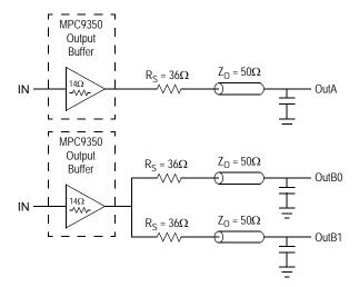
Figure 4. Single versus Dual Transmission Lines
