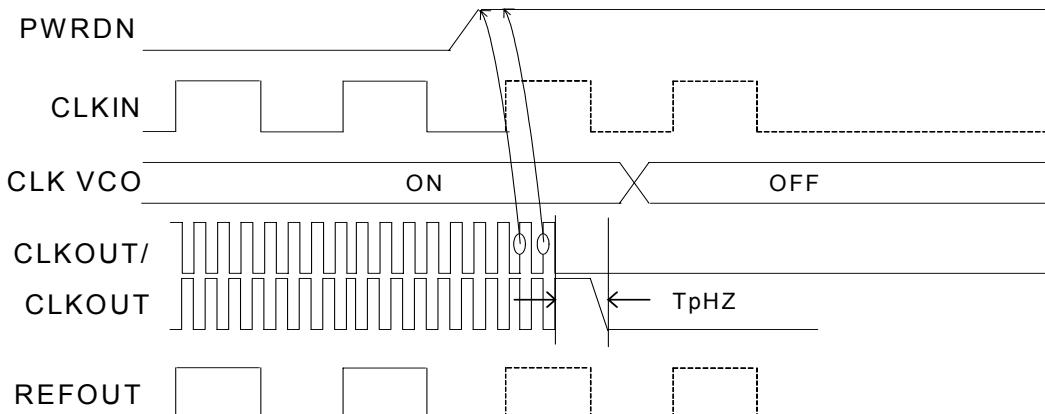
CLKOUT is driven differentially when PWRDWN# is de-asserted unless the CLKOUT is disabled through the SMBus register bit.
