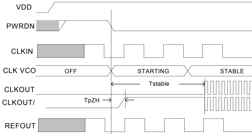
CLKIN must have a stable clock input when PWRDN is de-asserted. If CLKIN starts after PWRDN is de-asserted then  $T_{stable}$  specification applies to when CLKIN is ON. If CLKIN is full ON before PWRDN is de-asserted then the  $T_{stable}$  specification applies.
