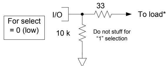
\*Note: Do not use a TTL load. This will overcome the  $10\text{k}\Omega$  pull-down and force the input to a logic 1.
