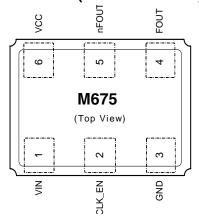
Figure 1: Pin Assignment
