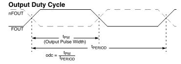
Figure 4: Output Duty Cycle
