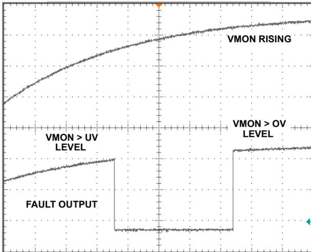
FIGURE 6. **V<sub>MONITOR</sub>** RISING TO FAULT
