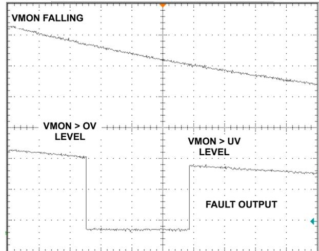
FIGURE 7. **V<sub>MONITOR</sub>** FALLING TO FAULT
