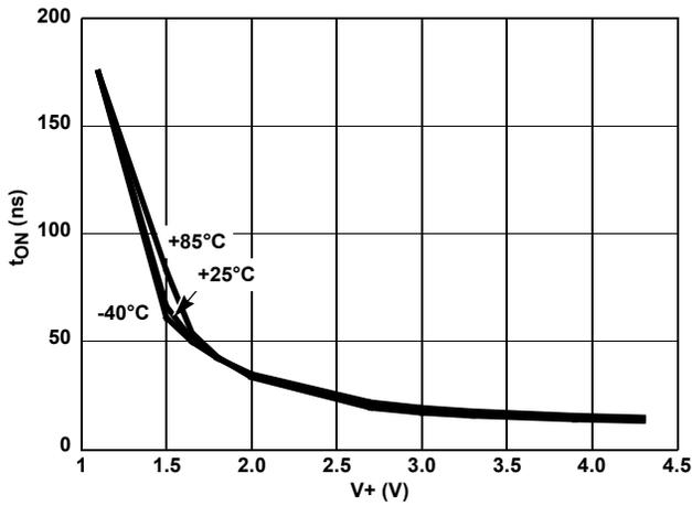
FIGURE 15. TURN - ON TIME vs SUPPLY VOLTAGE
