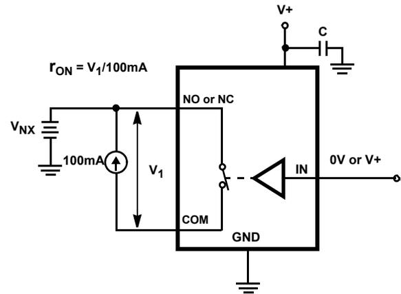
FIGURE 5.  $r_{ON}$  TEST CIRCUIT
