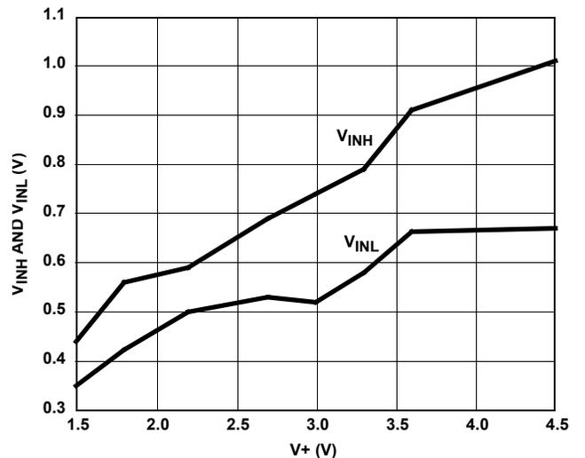
FIGURE 14. DIGITAL SWITCHING POINT vs SUPPLY VOLTAGE
