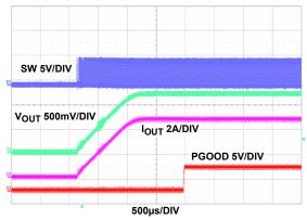
FIGURE 19. SOFT-START WITH 5A LOAD PWM MODE, V<sub>IN</sub> = 5V, V<sub>OUT</sub> = 1.2V, I<sub>OUT</sub> = 5A, C<sub>OUT</sub> =  $2x22\mu$ F CERAMIC CAPACITORS, C<sub>IN</sub> =  $100\mu$ F POSCAP +  $2x22\mu$ F CERAMIC CAPACITORS
