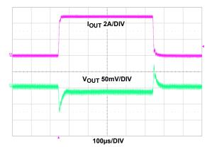
FIGURE 17.  $V_{IN}$  = 5V,  $V_{OUT}$  = 3.3V,  $I_{OUT}$  = 0 TO 5A,  $f_{SW}$  = 3MHz,  $C_{OUT}$  = 2x22µF CERAMIC CAPACITORS
