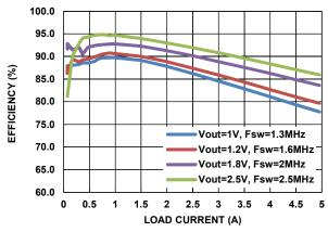
FIGURE 4. EFFICIENCY  $\rm T_A$  = +25 °C,  $\rm V_{IN}$  = 3.3V PFM MODE
