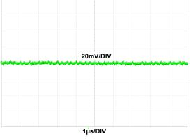
FIGURE 12.  $V_{IN}$  = 3.3V,  $V_{OUT}$  = 2.5V,  $I_{OUT}$  = 0A,  $f_{SW}$  = 2.5MHz,  $C_{OUT}$  = 2x22µF CERAMIC CAPACITORS
