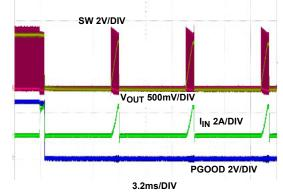
FIGURE 25. OUTPUT SHORT-CIRCUIT PROTECTION, HICCUP MODE
