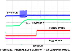
IGURE 23. PREBIAS SOFT-START WITH 0A LOAD PFM MODE, V<sub>IN</sub> = 5V, V<sub>OUT</sub> = 1.2V, I<sub>OUT</sub> = 0A, C<sub>OUT</sub> = 2x22µF CERAMIC CAPACITORS, C<sub>IN</sub> = 100µF POSCAP + 2x22µF CERAMIC CAPACITORS
