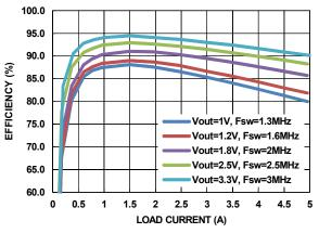
FIGURE 7. EFFICIENCY  $T_A = +25^{\circ}C$ ,  $V_{IN} = 5V$  PWM MODE
