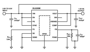
FIGURE 1. TYPICAL APPLICATION DIAGRAM AT  $5_{\mbox{VIN}}, \mbox{1.2V}_{\mbox{OUT}}, \mbox{1.6MHz} \mbox{ f}_{\mbox{SW}}, \mbox{5A}$
