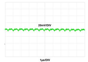
FIGURE 11.  $V_{IN}$  = 5V,  $V_{OUT}$  = 1.2V,  $I_{OUT}$  = 5A,  $f_{SW}$  = 1.6MHz,  $C_{OUT}$  = 2x22µF CERAMIC CAPACITORS
