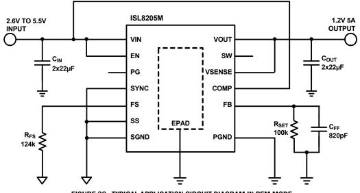
FIGURE 38. TYPICAL APPLICATION CIRCUIT DIAGRAM IN PFM MODE
