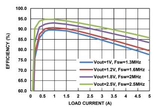
FIGURE 6. EFFICIENCY  $T_A = +25 \degree C$ ,  $V_{IN} = 3.3V PWM MODE$
