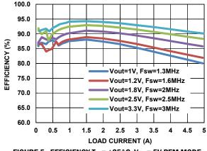
FIGURE 5. EFFICIENCY  $T_A = +25 \degree C$ ,  $V_{IN} = 5V$  PFM MODE
