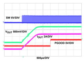
FIGURE 21. SOFT-START WITH 5A LOAD PFM MODE, V<sub>IN</sub> = 5V, V<sub>OUT</sub> = 1.2V, I<sub>OUT</sub> = 5A, C<sub>OUT</sub> = 2x22 $\mu$ F CERAMIC CAPACITORS, C<sub>IN</sub> = 100 $\mu$ F POSCAP + 2x22 $\mu$ F CERAMIC CAPACITORS
