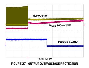
**Power Loss**  $T_A = +25$ °C,  $C_{IN} = 100\mu$ F POScap + 22 $\mu$ F ceramic capacitors,  $C_{OUT} = 2x22\mu$ F ceramic capacitors.
