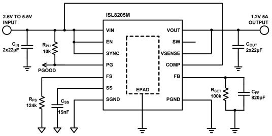
FIGURE 37. COMPLETE APPLICATION CIRCUIT DIAGRAM
