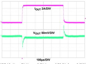
FIGURE 16. VIN = 5V, VOUT = 2.5V, IOUT = 0 TO 5A,  $f_{SW}$  = 2.5MHz,  $C_{OUT}$  = 2x22  $\mu F$  CERAMIC CAPACITORS
