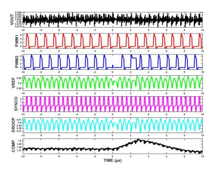
Figure 70. f<sub>SW</sub> = 1MHz, trigger V<sub>OUT</sub> ±20mV
