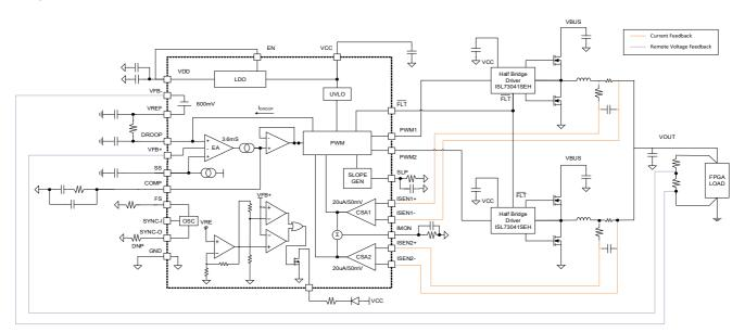
Figure 69. DUT SEE Irradiation Setup
