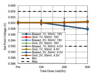
Figure 63. Set Point Voltage vs TID
