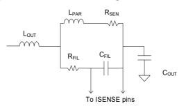
Figure 51. R<sub>SEN</sub> Parasitic Inductance Compensation RC Circuit
