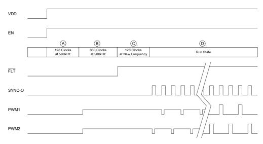
Figure 48. Start-Up Timing Diagram (R<sub>SYNC-O</sub> = 100kΩ)
