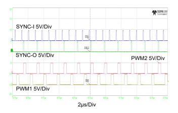
Figure 43. SYNC (V<sub>DD</sub> = 5V, P<sub>VIN</sub> = 12V, RSYNC-O = 100k $\Omega$  to VCC, FSYNC-I = 1.15MHz)
