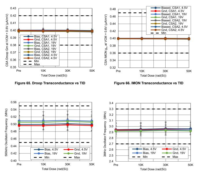
Figure 67. Oscillator Frequency vs TID (f<sub>OSC</sub> = 0.5MHz)
