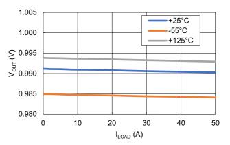
Figure 9. Load Regulation for Various Temperatures (V<sub>IN</sub> = 12V)
