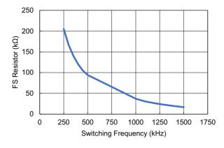
Figure 50. R<sub>FS</sub> vs Frequency
