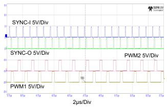
Figure 44. SYNC (V<sub>DD</sub> = 5V,  $P_{VIN}$  = 12V, RSYNC-O = 100k $\Omega$ to GND, FSYNC-I= 1.15MHz)
