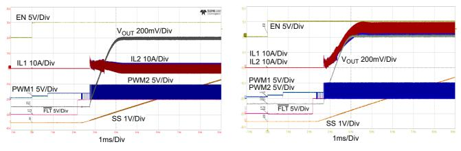
Figure 29. Start-Up with EN  $(P_{VIN} = V_{DD} = 12V, I_{LOAD} = 0A$
