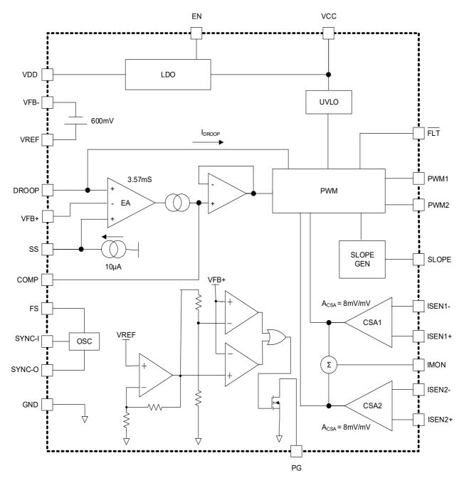
Figure 5. Block Diagram
