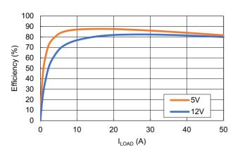
Figure 19. Conversion Efficiency for Various V<sub>IN</sub> (f<sub>SW</sub> = 500kHz, Tested on the ISL73847MDEMO1Z)
