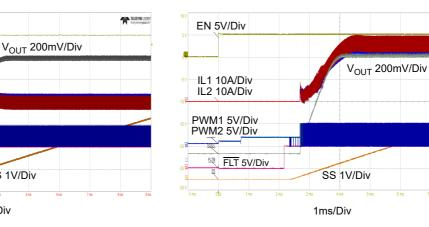
Figure 31. Start-Up with EN  $(P_{VIN} = V_{DD} = 13.2V, I_{LOAD} = 0A$
