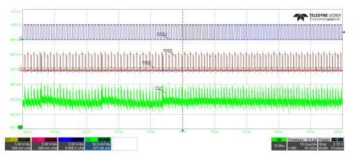
Figure 49. Switching between Internal Oscillator and External Oscillator on SYNC-I (External clock frequency changed from 1MHz to 1.15MHz)
