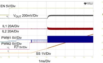
Figure 37. Pre-Biased Start-Up  $(V_{DD} = 4.62V, P_{VIN} = 12V, I_{LOAD} = 0A, Vpre-bias = 900mV$
