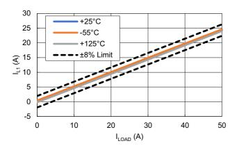
Figure 15. Phase 1 Current Share vs Temperature (V<sub>IN</sub> = 5V)
