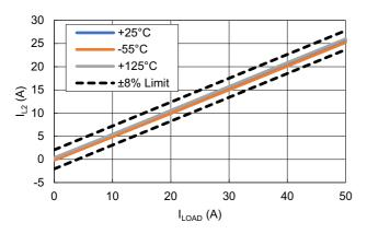
Figure 17. Phase 1 Current Share vs Temperature (V<sub>IN</sub> = 12V)
