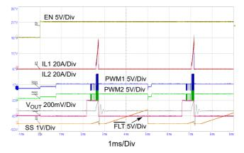
Figure 41. Start-Up with a Short ( $P_{VIN} = V_{DD} = 5V$ )
