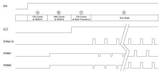
Figure 47. Start-Up Timing Diagram (R<sub>SYNC-O</sub> = OPEN)
