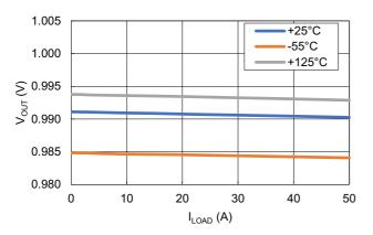
Figure 8. Load Regulation for Various Temperatures (V<sub>IN</sub> = 5V)
