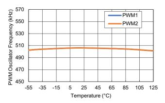
Figure 22. PWMx Frequency vs Temperature (V<sub>IN</sub> = 5V,  $I_{LOAD} = 50A$ )
