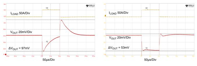
Figure 55. Transient Response without Droop Regulation
