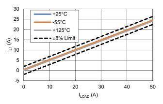
Figure 18. Phase 2 Current Share vs Temperature (V<sub>IN</sub> = 12V)
