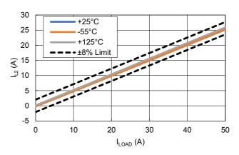
Figure 16. Phase 2 Current Share vs Temperature (V<sub>IN</sub> = 5V)
