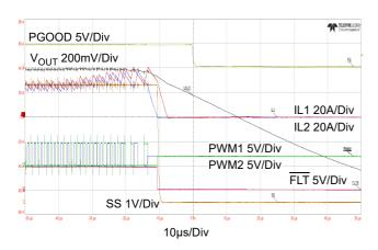
Figure 39. Overcurrent Protection (P<sub>VIN</sub> = 12V, V<sub>DD</sub> = 5V)
