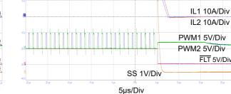
Figure 35. Shutdown with EN  $(P_{VIN} = V_{DD} = 12V, I_{LOAD} = 0A$
