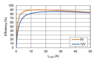
Figure 20. Conversion Efficiency for Various V<sub>IN</sub> ( $f_{SW}$  = 250kHz, Tested on the ISL73847MDEMO1Z), L<sub>OUT</sub> = 450nH per phase, C<sub>OUT</sub> = 5.28mF per phase, C<sub>COMP</sub> = 15nF, C<sub>DROOP</sub> = 100nF, R<sub>FS</sub> = 205kΩ
