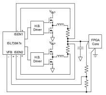
Figure 1. FPGA Core Power Supply Application
