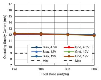
Figure 59. Operating Supply Current vs TID
