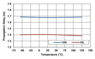
Figure 13. Input Logic Threshold vs Temperature
