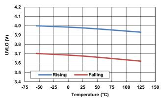
Figure 7.  $V_{DRV}$  Undervoltage Lockout Threshold
