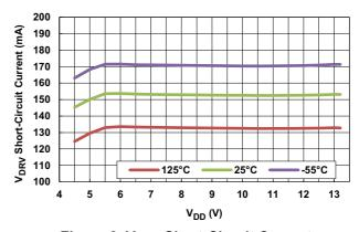
Figure 8. V<sub>DRV</sub> Short-Circuit Current vs Temperature
