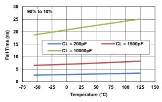
Figure 15. Output Fall Times vs Temperature
