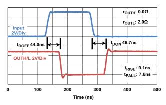
Figure 12. Input Bar Propagation Delay
