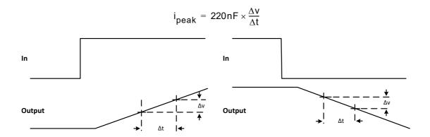
Figure 4. Peak Source/Sink Measurement
