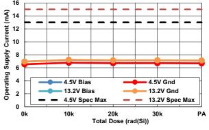
Figure 21. Operating Supply Current vs TID
