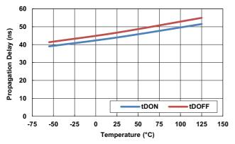
Figure 11. Input Bar Propagation Delay vs Temperature
