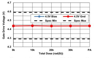
Figure 22.  $V_{DRV}$  Voltage vs TID ( $V_{DD} = 4.5V$ )
