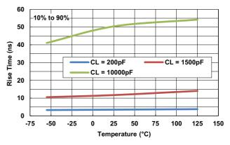
Figure 14. Output Rise Times vs Temperature
