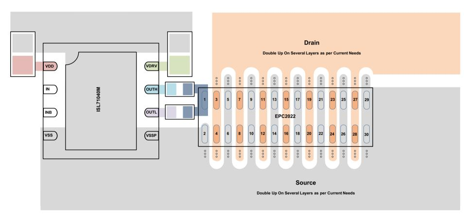
Figure 18. PCB Layout Recommendation
