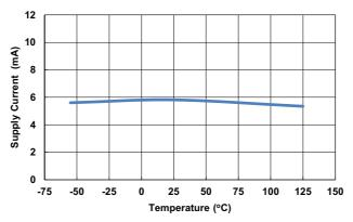
Figure 17. Operating Supply Current
