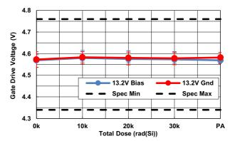
Figure 23. V<sub>DRV</sub> Voltage vs TID (V<sub>DD</sub> = 13.2V)
