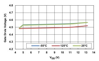
Figure 2. V<sub>DRV</sub> Line Regulation vs Temperature
