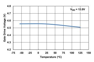
Figure 6. V<sub>DRV</sub> vs Temperature
