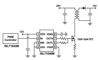
Figure 1. Typical Flyback Power Supply Application
