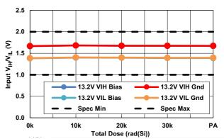
Figure 25.  $V_{IH}/V_{IL}$  Level vs TID ( $V_{DD} = 13.2V$ )
