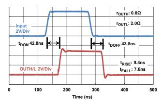
Figure 10. Input Propagation Delay
