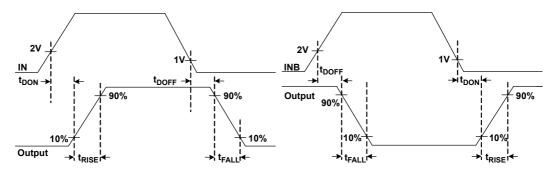
Figure 3. Timing Diagram, OUTH and OUTL Tied Together
