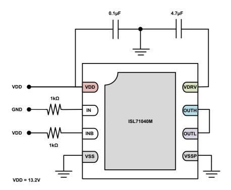
Figure 19. Irradiation Bias Configuration for the ISL71040M
