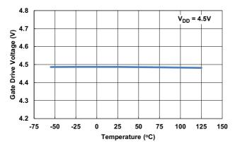
Figure 5. V<sub>DRV</sub> vs Temperature
