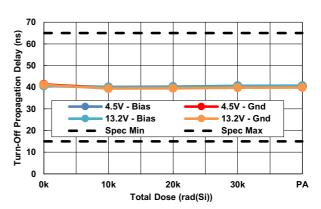
Figure 27. t<sub>DOFF</sub> vs TID
