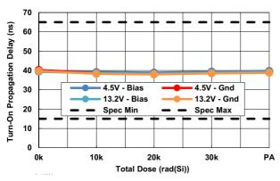
Figure 26. t<sub>DON</sub> vs TID
