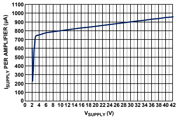
FIGURE 26. SUPPLY CURRENT vs SUPPLY VOLTAGE
