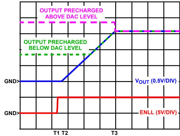
FIGURE 7. SOFT-START WAVEFORMS FOR ISL6563-BASED MULTIPHASE CONVERTER
