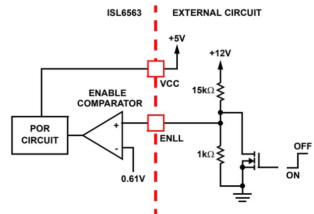
FIGURE 6. START-UP COORDINATION USING THRESHOLD-SENSITIVE ENABLE (ENLL) PIN
