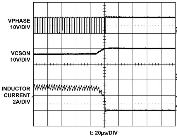
FIGURE 11. BATTERY REMOVAL
