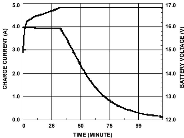
FIGURE 3. BATTERY CHARGE V-I CHARACTERISTICS
