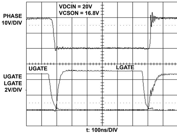
FIGURE 13. SWITCHING WAVEFORMS AT CONSTANT CHARGE CURRENT MODE
