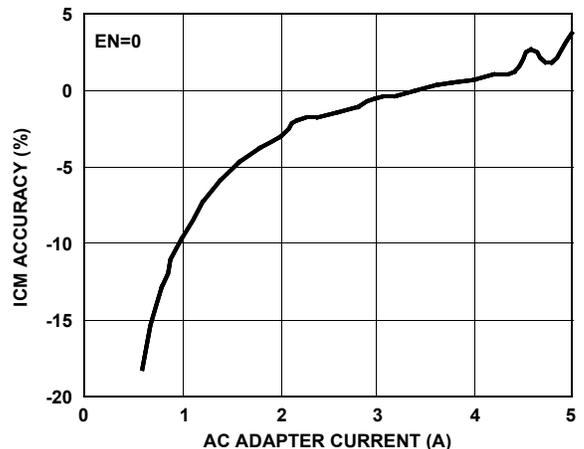
FIGURE 6. ICM ACCURACY vs AC ADAPTER CURRENT
