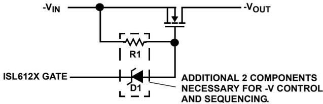
D1 necessary to prevent premature turn-on. R1 is used to hold FET Vgs = 0V until D1 Vz is overcome. R1 value can be changed to adjust -V ramp rates. Choose an R1 value between 4MW and 10MW initially, and fine-tune resistor value for the particular need.
