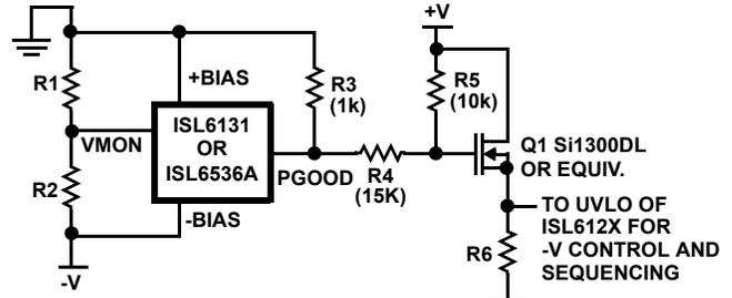
R1 and R2 define -V UVLO level. R3 ensures supervisor (ISL6131 or ISL6536A) PGOOD pull-up. R4 and R5 provide Q1 gate bias between 0V and +V to 0V (resistor values suitable for -V = -5V and +V = +3.3V).
