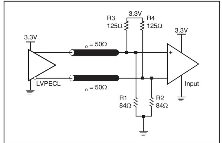
Figure 1B. 3.3V LVPECL Output Termination
