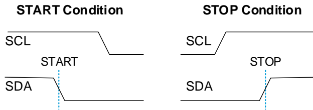
Figure 10. START and STOP Condition Waveform
